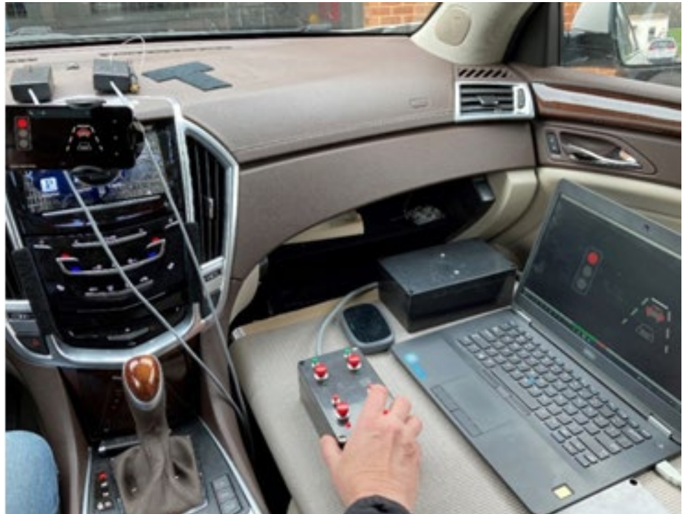
Figure 2. In-vehicle signal and display control system for Exploring the Effects of Vehicle Automation and Cooperative Messaging on Mixed Fleets Eco-Drive project.
