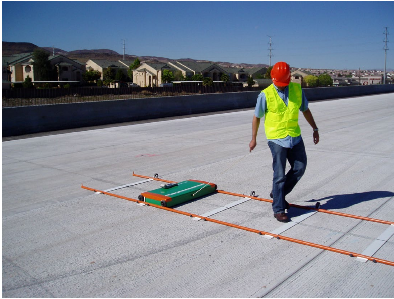
Figure 4. Photo. Testing a pavement transverse joint using an MIT scanning device.
