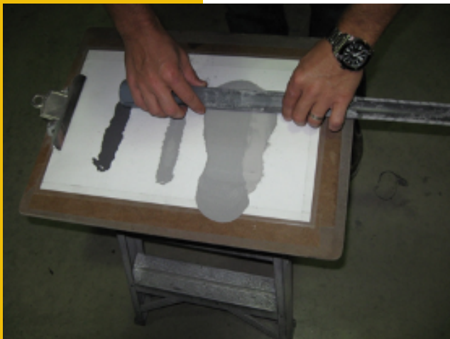
A clipboard showing samples of fly ash before and after electrostatic separation to reduce the amount of carbon in fly ash. The dark gray/black contains the carbon removed from the fly ash, the medium gray is the fly ash entering the separation system, and the light gray is the fly ash product to be used in concrete.
