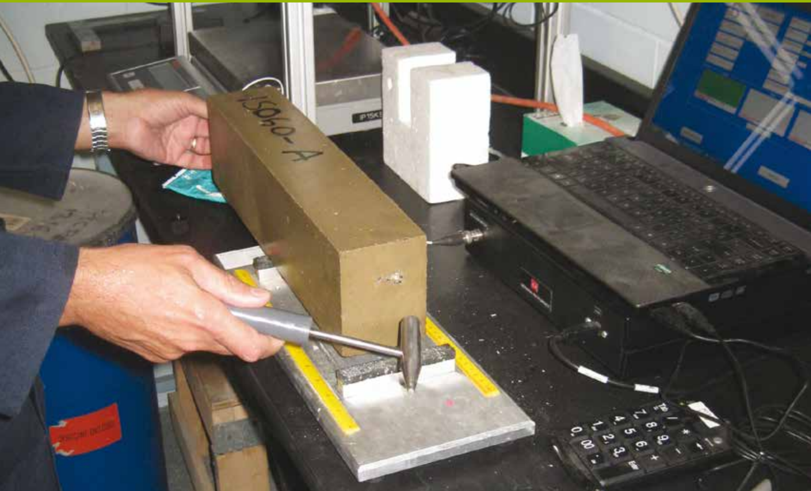
Figure 6. Photo: Laboratory research methods include dynamic modulus of concrete with the measurement of fundamental resonant frequency. Source: FHWA.
