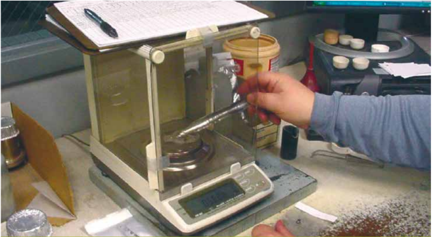
Figure 3. Photo: A researcher determines the mass of a specimen on a laboratory balance. Source: FHWA.
