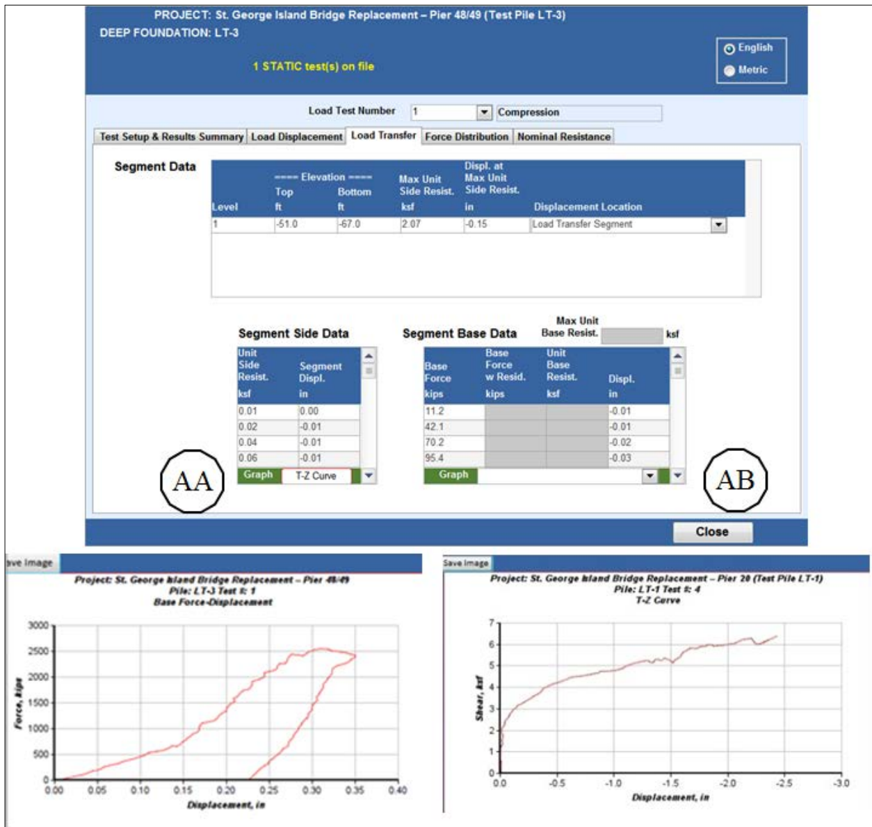
Figure 23. Static Load Test Graphics Options within Load Tab test. Load Transfer tab.
