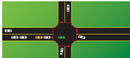
An AIM simulation, which shows virtual and real vehicles at an intersection. White vehicles have a reservation to enter the intersection; yellow vehicles do not. The green vehicle is a proxy, representing the real-world location of the autonomous vehicle.
