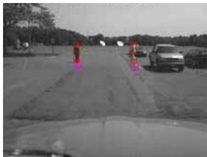
Visual output of the pedestrian-detection system as it recognizes crossing pedestrians.
