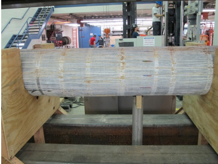
Figure 123. Photo. Stainless steel straps removed from south central side of cable mockup specimen.
