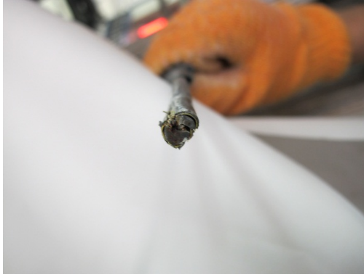
Figure 173. Photo. Crushed CMAS Zn 2 sensor.
