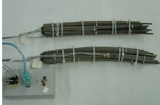
Figure 5. Photo. Wire bundles to be placed in corrosion chamber.
