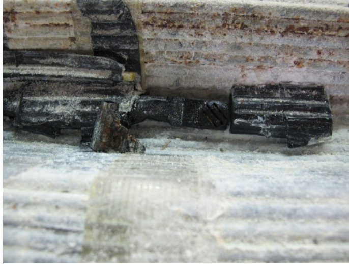
Figure 159. Photo. Precon HS2000V sensor 13 during cable dissection.
