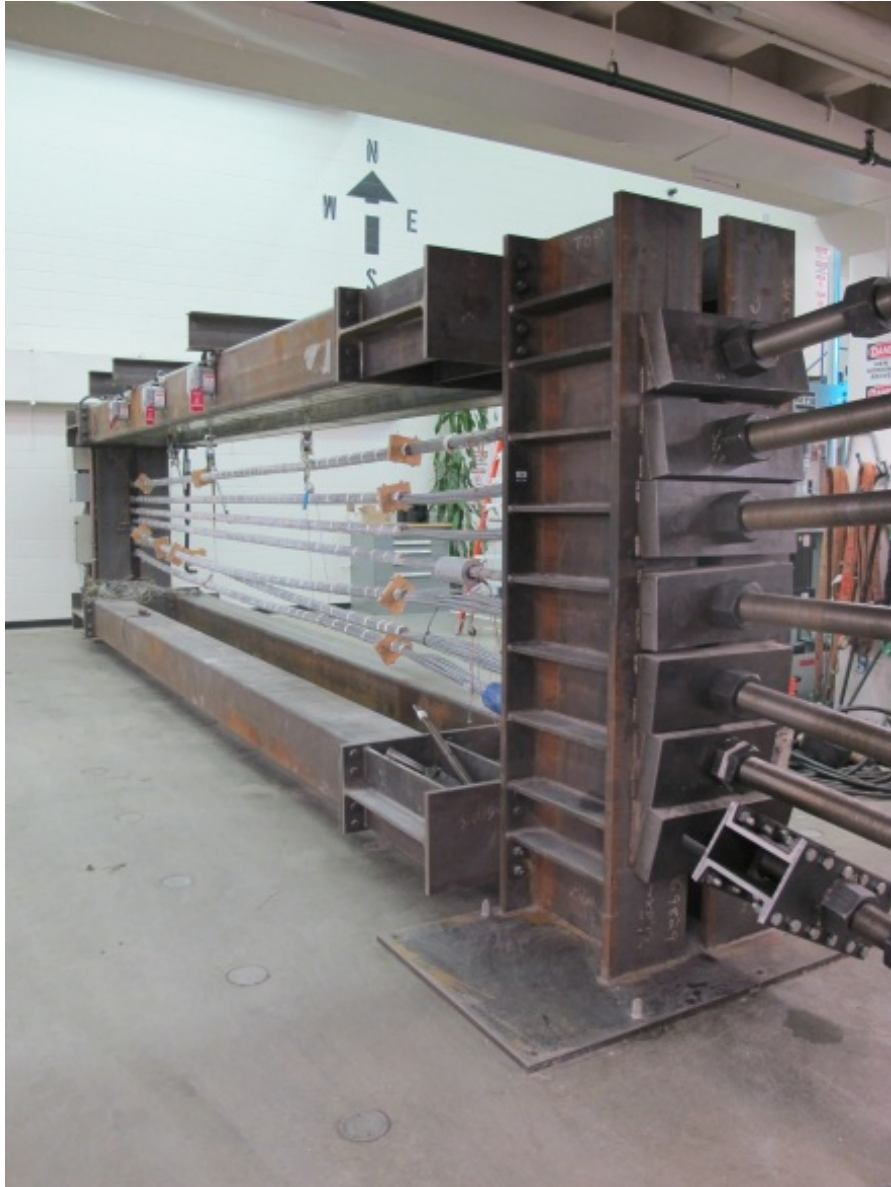
Figure 129. Photo. Completed cable deconstruction.
