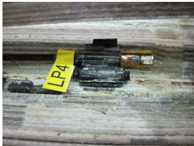
Figure 164. Photo. LPR sensor 4 during cable disassembly.
