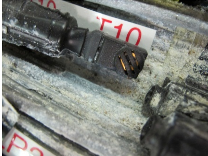
Figure 163. Photo. Precon HS2000V sensor 10 during cable dissection.
