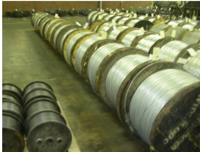
Figure 72. Photo. Wire coils to be used for the construction of the cable mockup (first row of coils).
