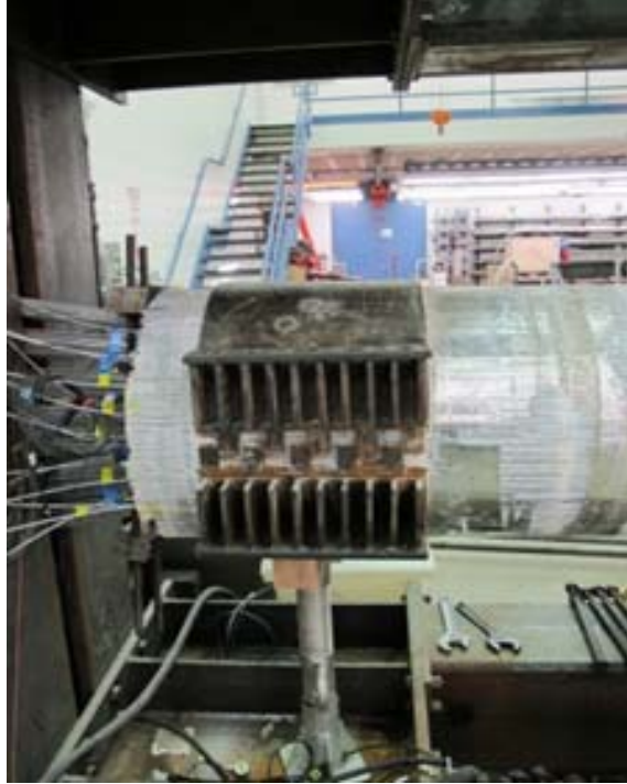
Figure 125. Photo. North side prior to cable band removal.
