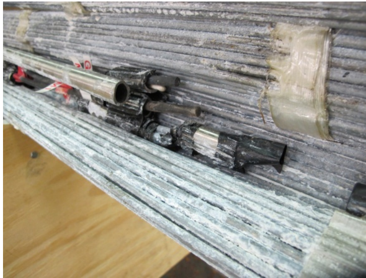
Figure 156. Photo. Sensors T1, BM1, and CMAS CS1.
