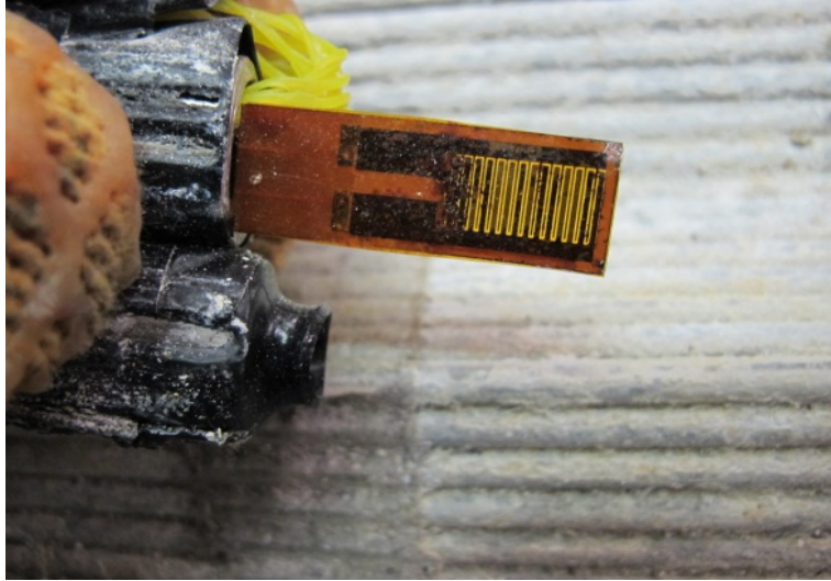
Figure 165. Photo. Close-up view of LPR sensor 4.
