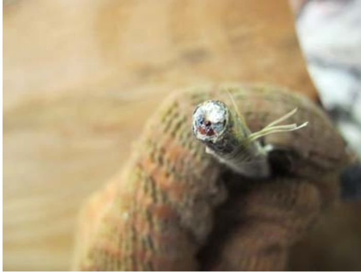
Figure 174. Photo. Heavy corrosion on BM sensor 7.
