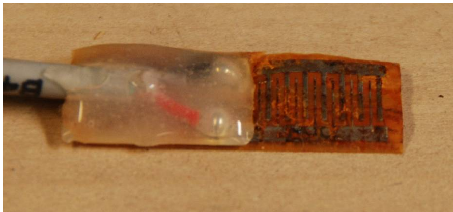
Figure 9. Photo. Corroded LPR sensor after 1 week test.
