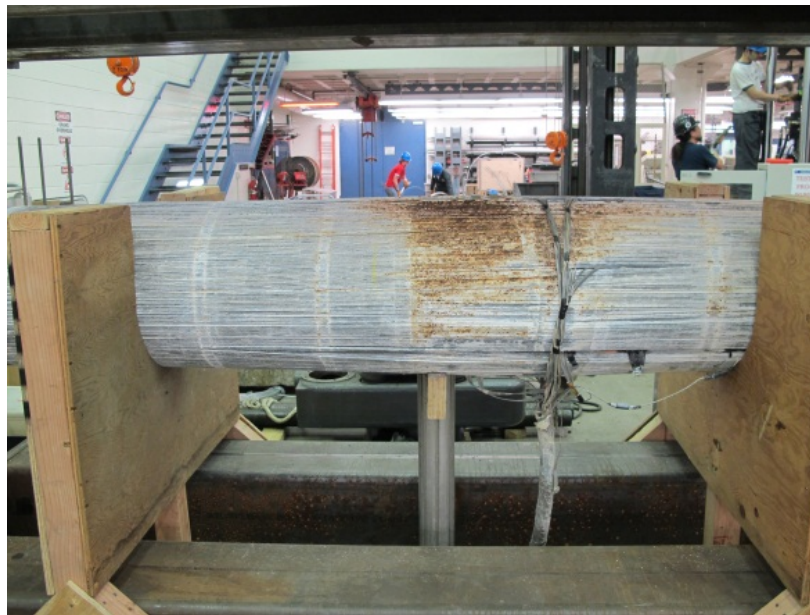
Figure 122. Photo. Stainless steel straps removed from north central side of cable mockup specimen.
