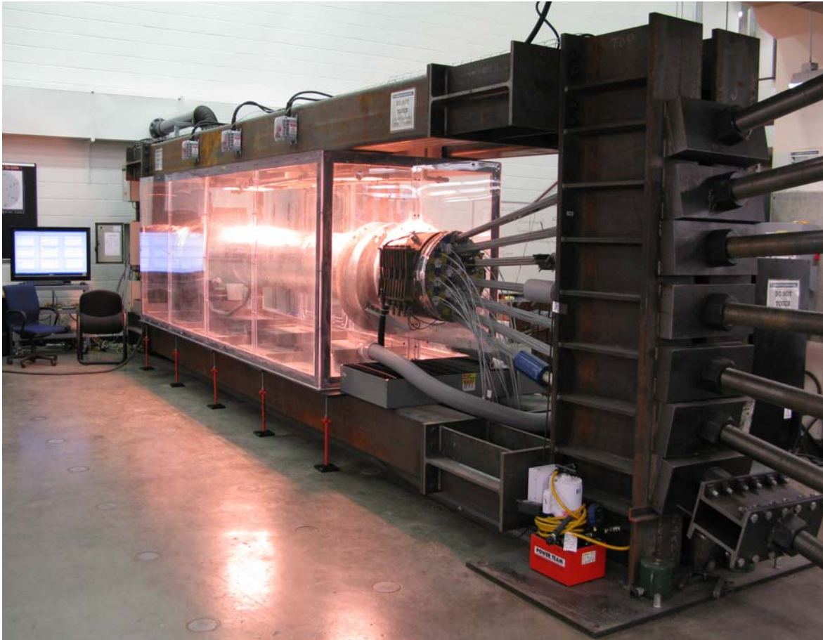
Figure 85. Photo. Cable specimen with environmental chamber.
