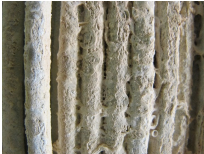
Figure 146. Photo. Close-up view of the product formed on the high-strength steel wires.
