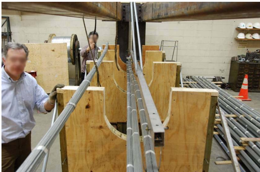
Figure 77. Photo. Lower strand assemblage.
