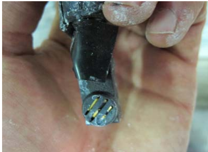
Figure 158. Photo. Close-up view of Precon HS2000V sensor 3 electrode.
