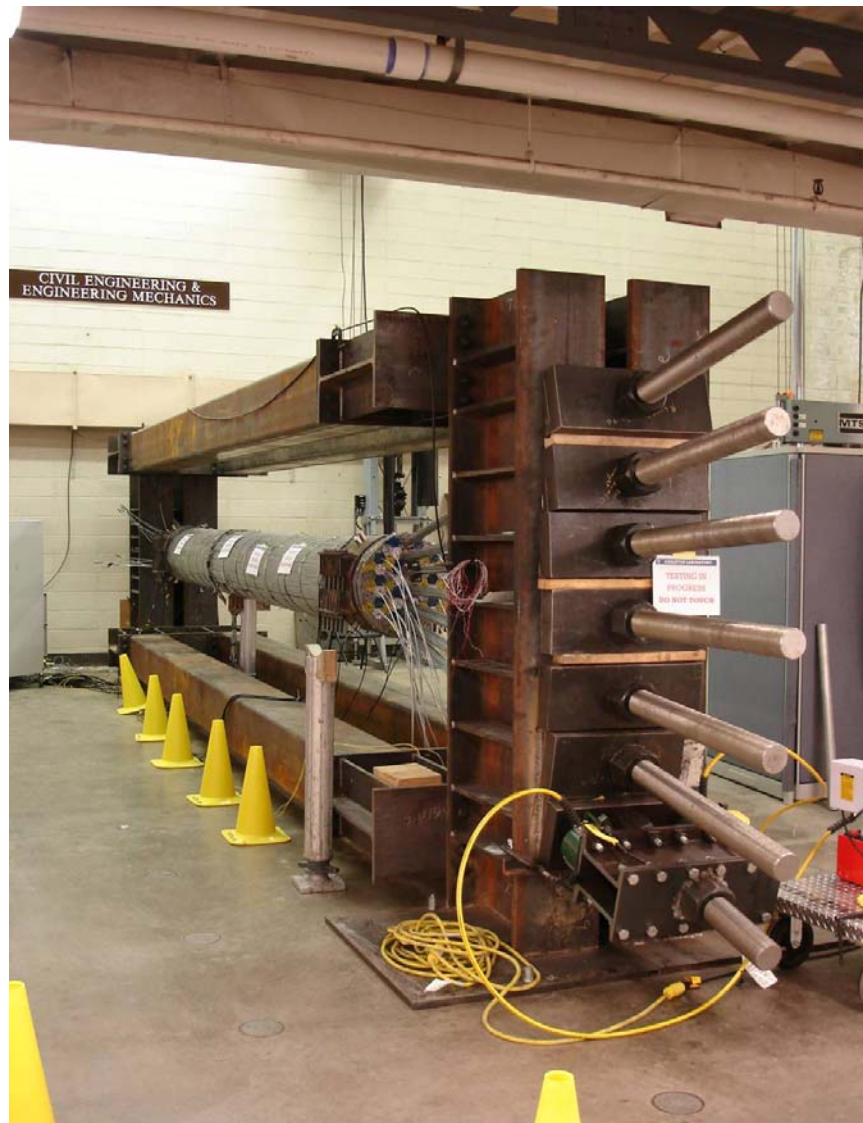
Figure 84. Photo. Cable mockup representative of a full-scale section of a suspension bridge cable.
