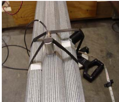
Figure 64. Photo. Mounted AE sensors.
