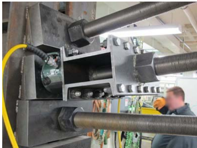
Figure 117. Photo. Jacking beam with hydraulic jacks secured into position.
