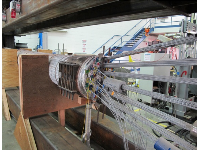
Figure 115. Photo. Disassembled environmental chamber with cable mockup specimen.
