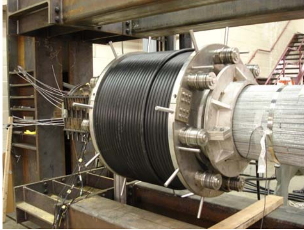
Figure 67. Photo. MMFM bobbin mounted on a cable mockup.
