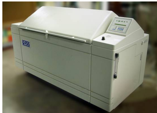
Figure 4. Photo. Q-fog cyclic corrosion tester.
