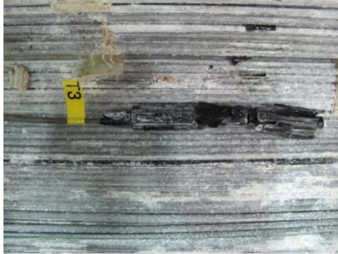
Figure 157. Photo. Precon HS2000V sensor 3 during cable disassembly.
