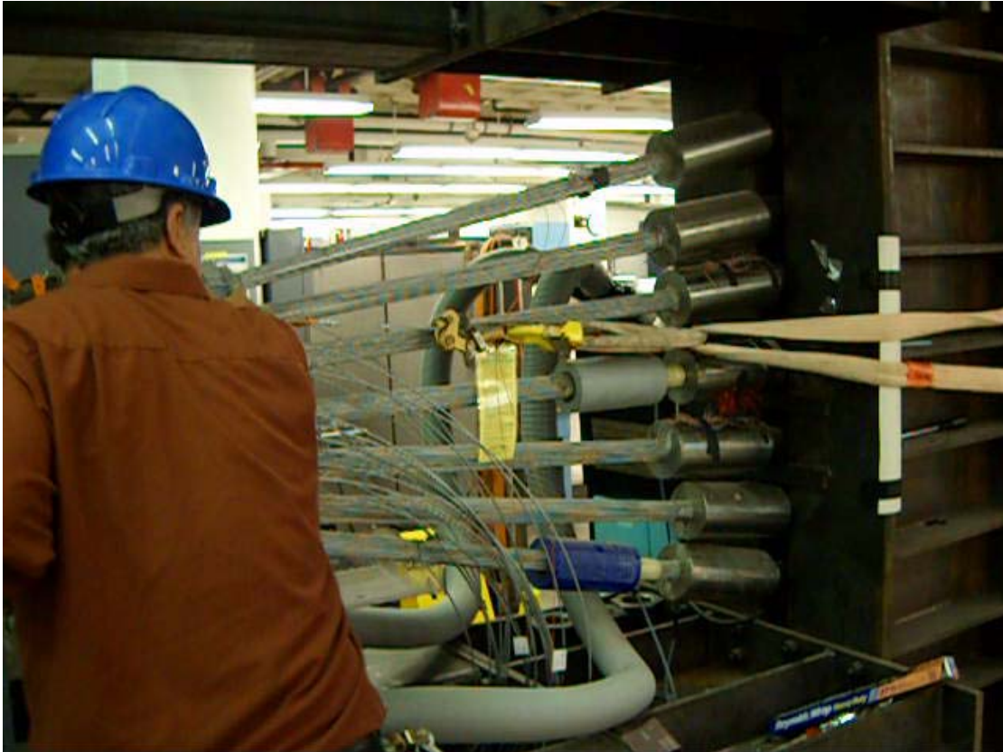
Figure 106. Photo. Mechanism to apply load to the prenotched wires.
