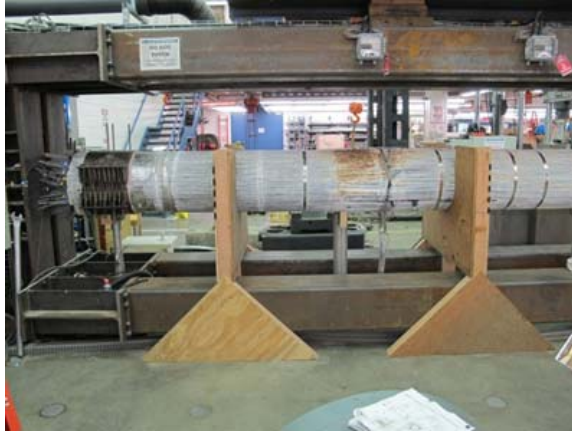
Figure 119. Photo. North end of cable mockup with stainless steel straps.
