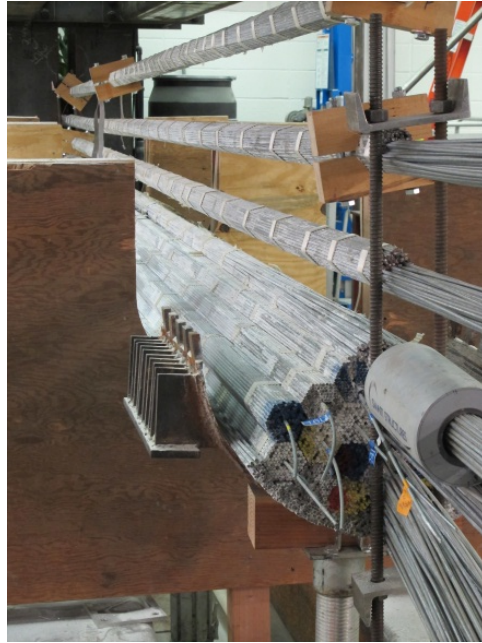
Figure 127. Photo. Cable specimen during disassembly.
