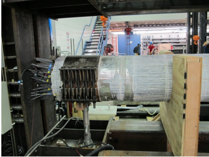
Figure 121. Photo. Stainless steel straps removed from north side of cable mockup specimen.
