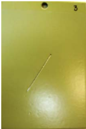
Figure 23. Photo. Progressive changes of IOZ/E/PU—type I in ALT, NW, and NWS.
