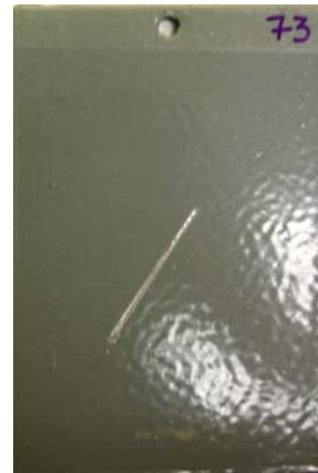
Figure 29. Photo. Progressive changes of ZnE/LE—type I in ALT, NW, and NWS.
