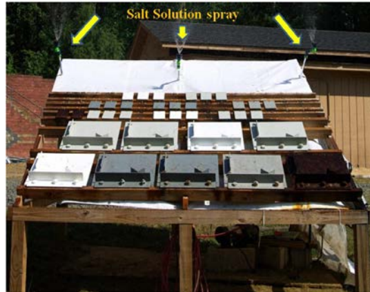
Figure 7. Photo. NWS rack at TFHRC.
