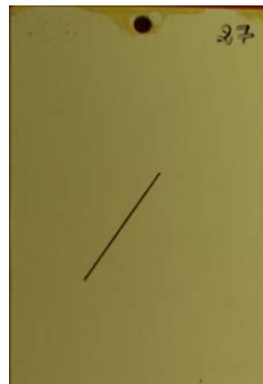
Figure 25. Photo. Progressive changes of MCU/E/F—type I in ALT, NW, and NWS.
