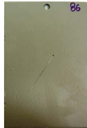
Figure 30. Photo. Progressive changes of HRCSA—type I in ALT, NW, and NWS.
