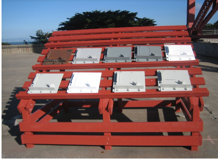
Figure 10. Photo. Type II panels deployed at GGB.
