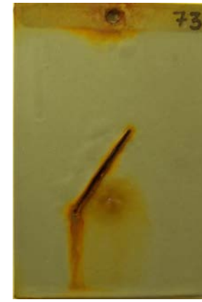
Figure 29. Photo. Progressive changes of ZnE/LE—type I in ALT, NW, and NWS.
