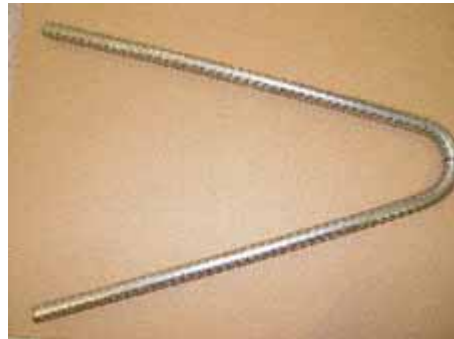
Figure 1. Photo. 2304 SS bar after bending.
