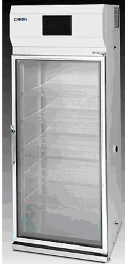
Figure 17. Photo. CARON ® environmental chamber for cyclic SAE J2334 tests.
