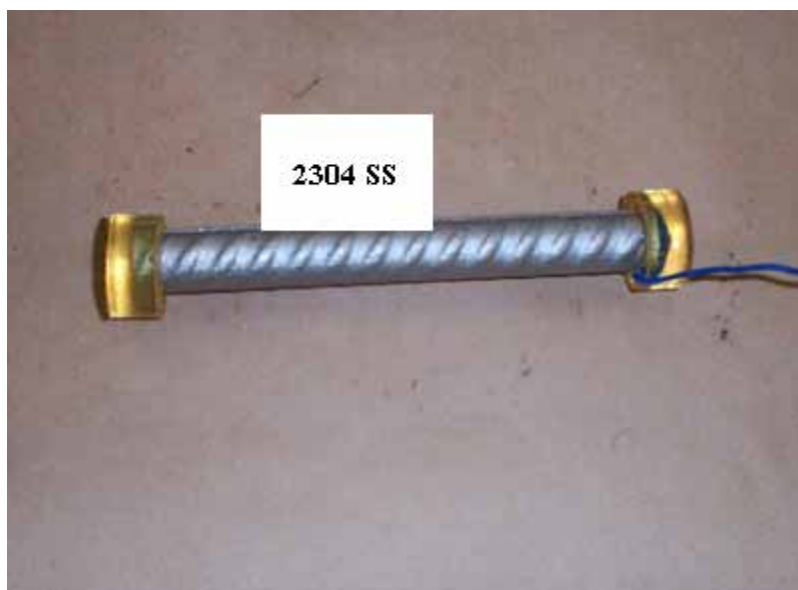
Figure 6. Photo. Straight as-received 2304 SS bar with epoxy-mounted ends and an electrical lead.
