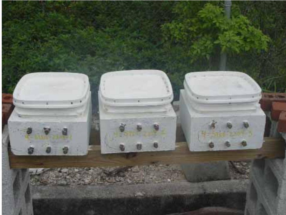
Figure 10. Photo. SDS specimens reinforced with 2304 SS under test.
