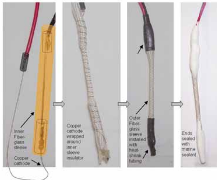
Figure 28. Photo. Completion of the cable sensor.
