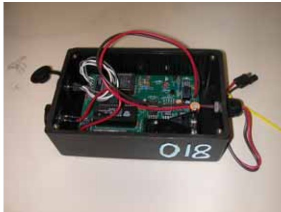
Figure 22. Photo. Data logger incorporating a ZRA.
