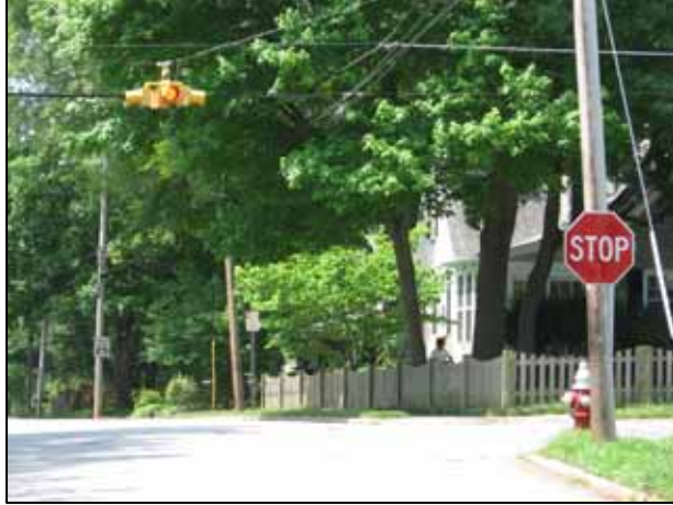
Figure 1. Photo. Example of Standard Overhead Flashing Beacon.
