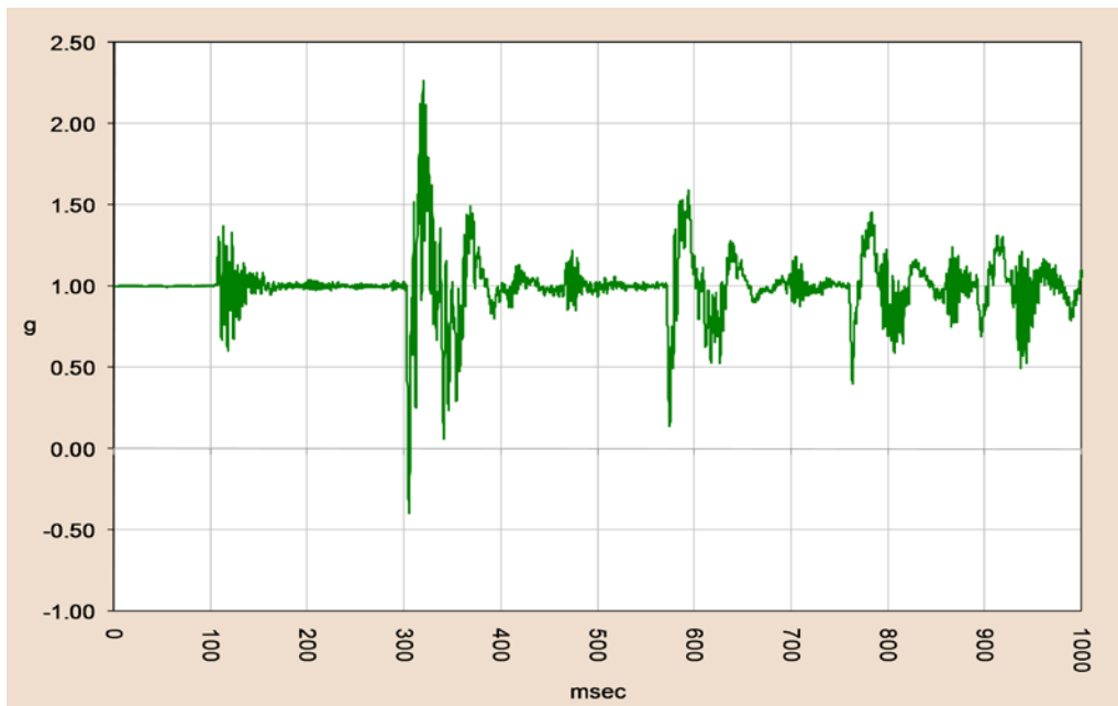
Figure 21. Graph. Raw accelerometer output from a JILS FWD impulse.
