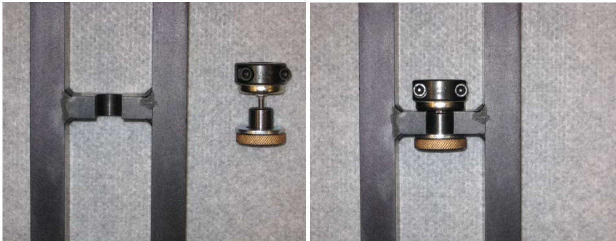
Figure 123. Photo. Attachment of a KUAB geophone adapter.
