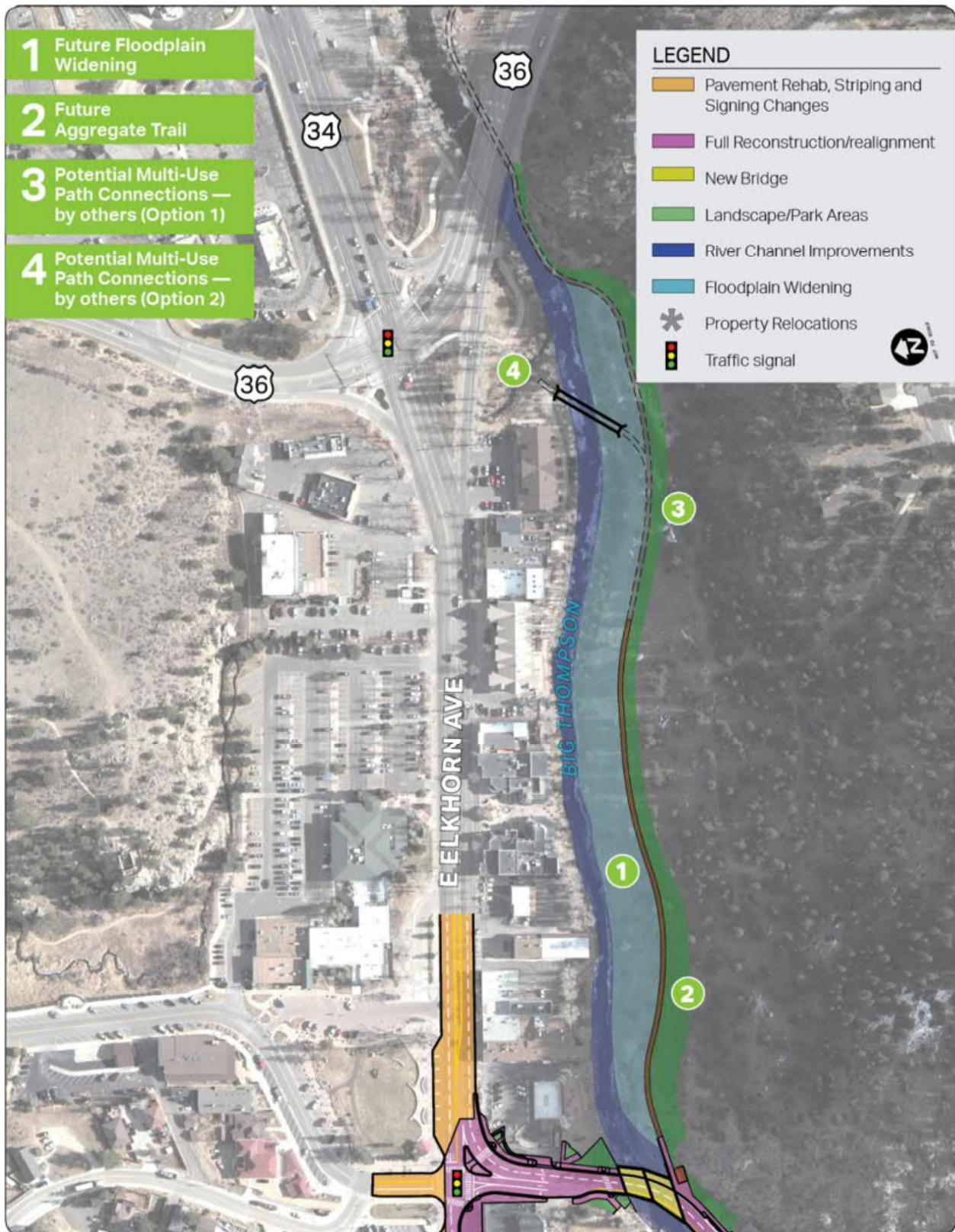
Figure 2-10: Downstream Channel Improvements
