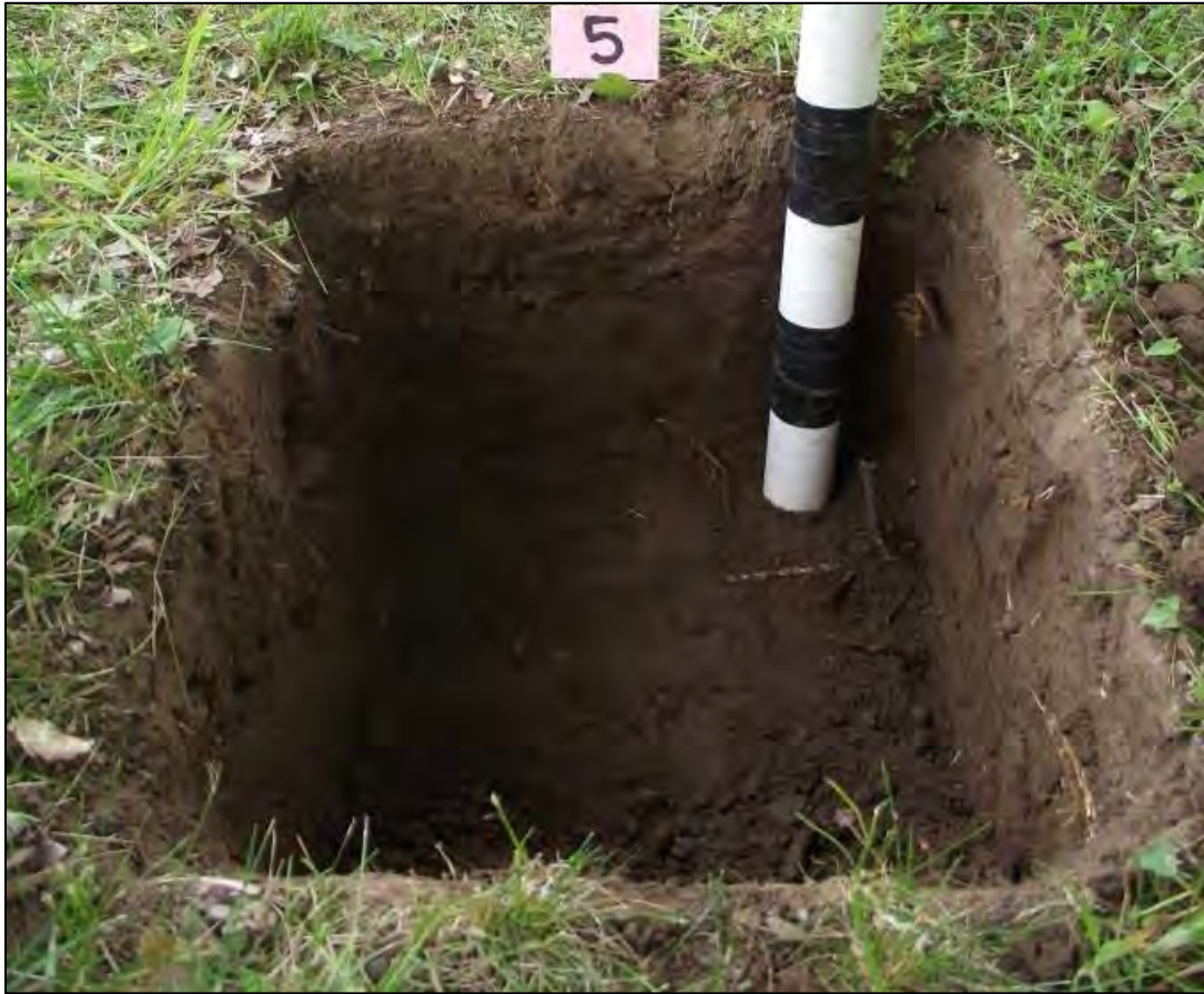
Figure 5. Soil Test Pit NE of the Bridge
