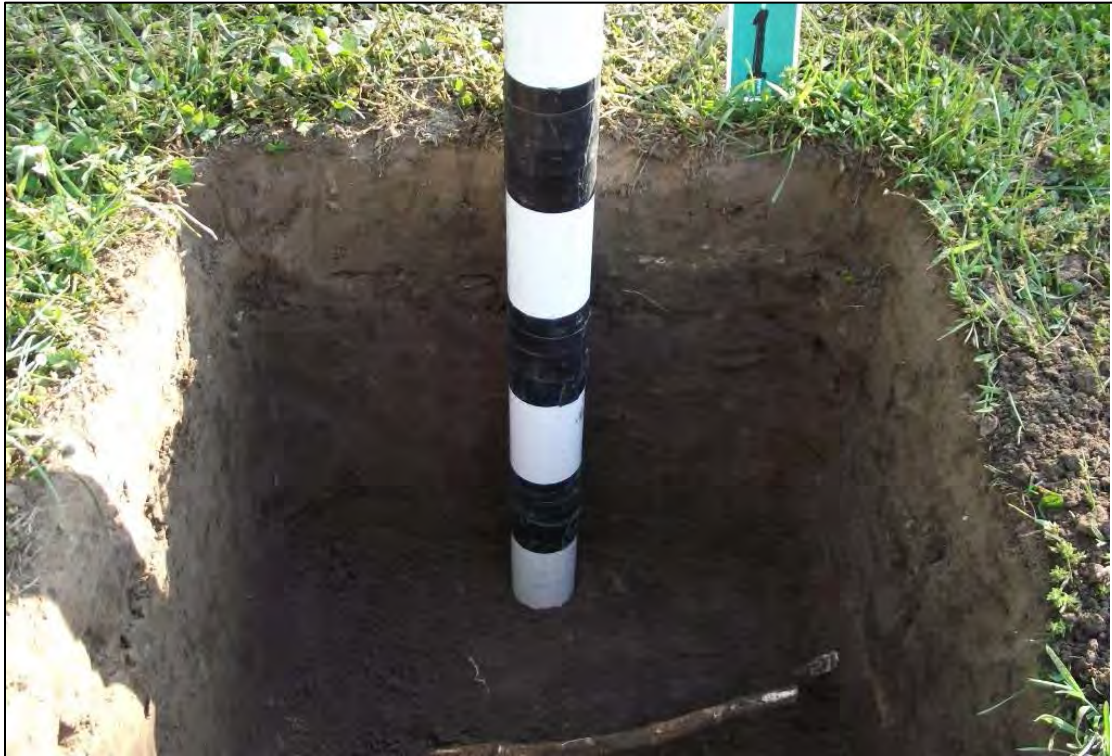
Figure 4. Soil Test Pit NW of the Bridge
