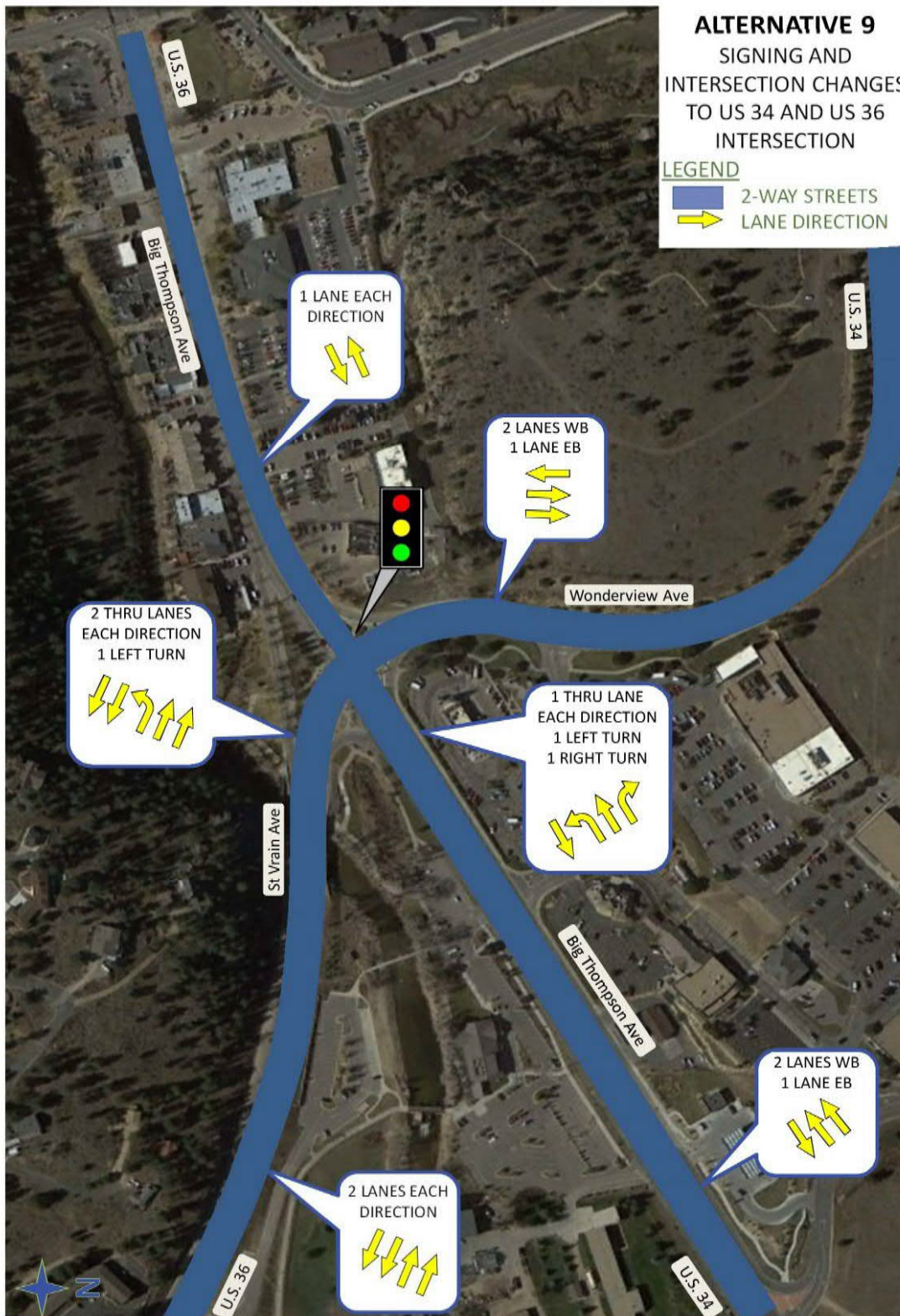
Figure A-12: Alternative 9 (Traffic Division, Signage/Intersection Modifications)
