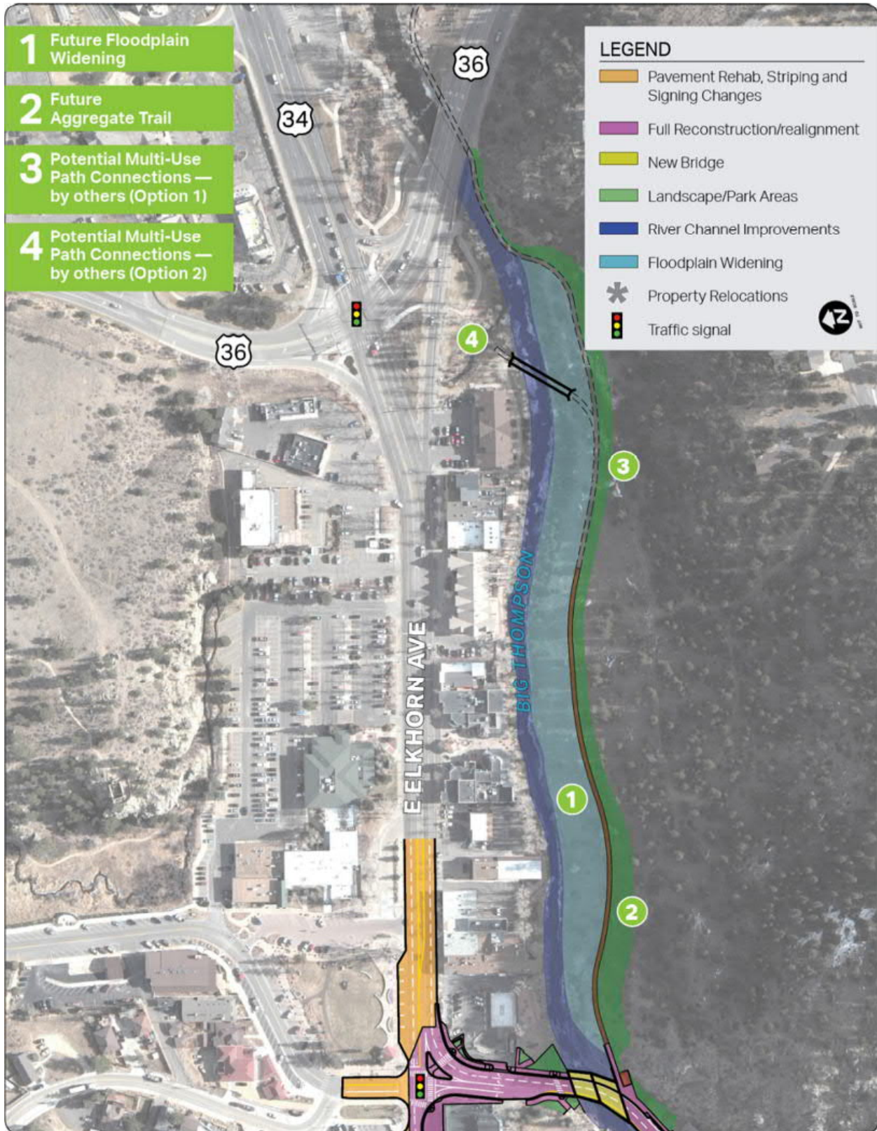
Figure 2-10: Downstream Channel Improvements
