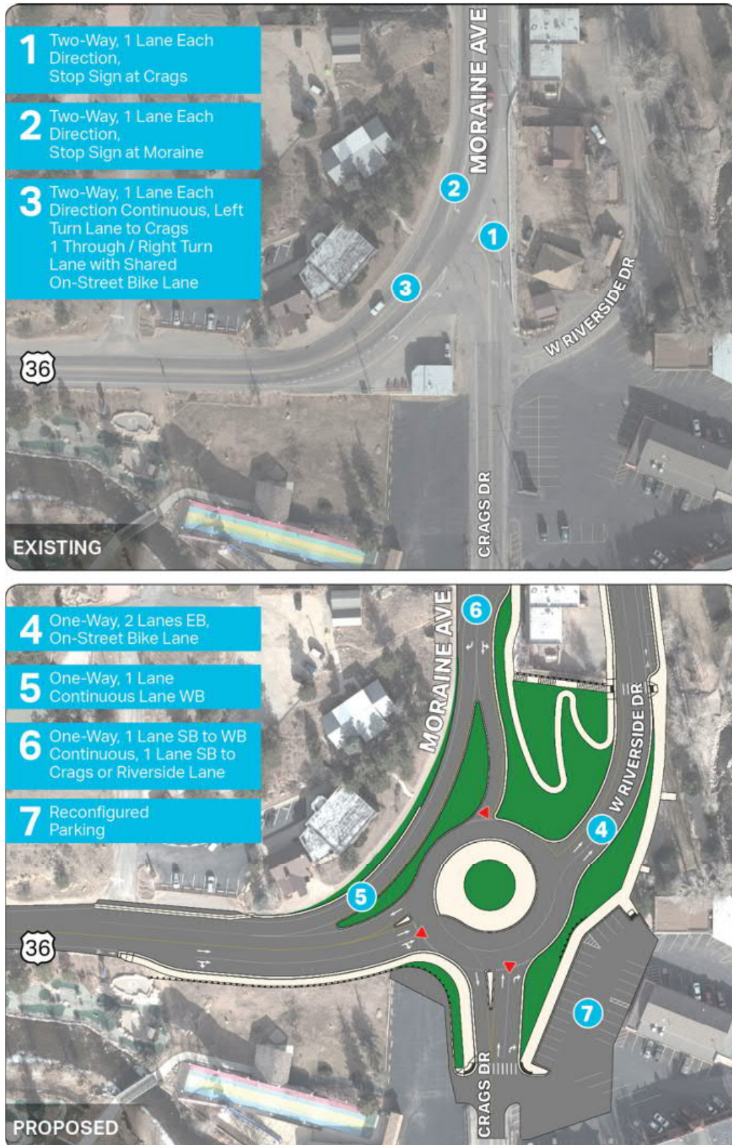
Figure 2-8: Existing and Proposed Moraine Avenue/Riverside Drive/Crags Drive (Roundabout Option)
