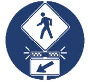
***A Rectangular Rapid Flashing Beacon (RRFB) is a pedestrian-actuated device that flashes in an alternating high-frequency pattern to alert drivers to a pedestrian using an uncontrolled, marked crosswalk.***
