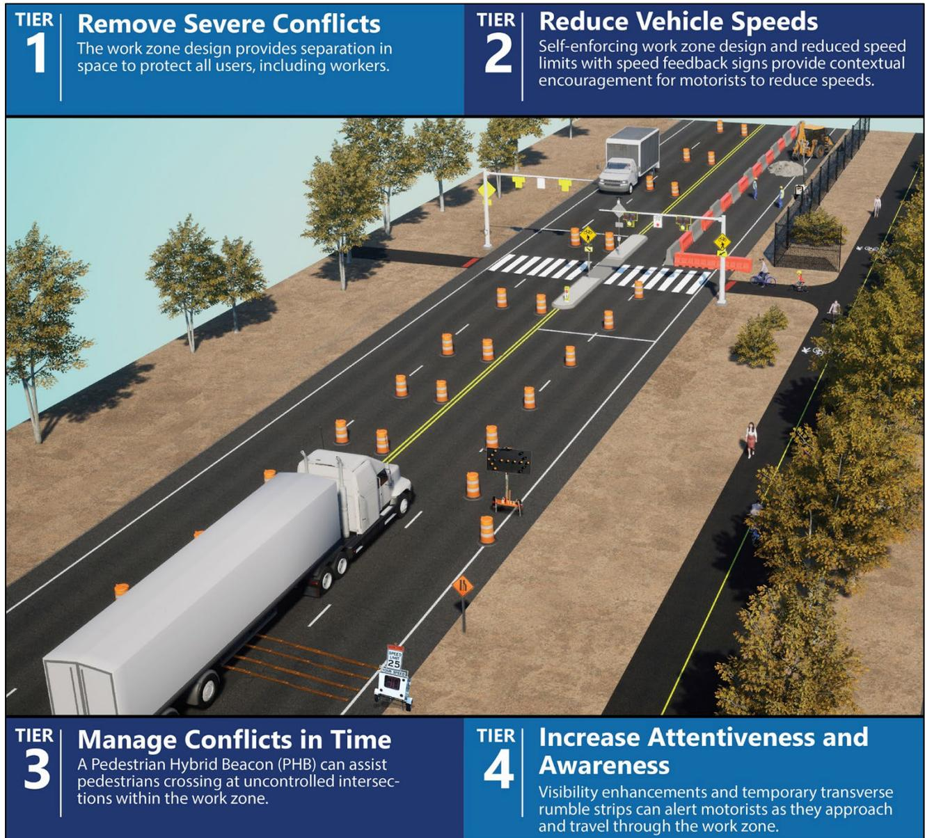
Figure 5. Example work zone layout with safety countermeasures that align with the *Safe System Roadway Design Hierarchy*. Source: FHWA
