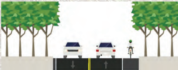
26-foot roadway with 10-foot lanes, 5-foot bicycle lane, and a 1-foot shoulder
