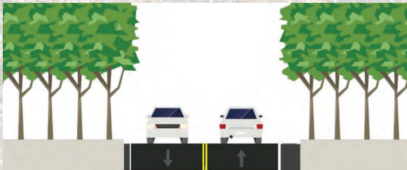
24-foot roadway with 10-foot lanes and a 1-foot shoulder and 3-foot shoulder
