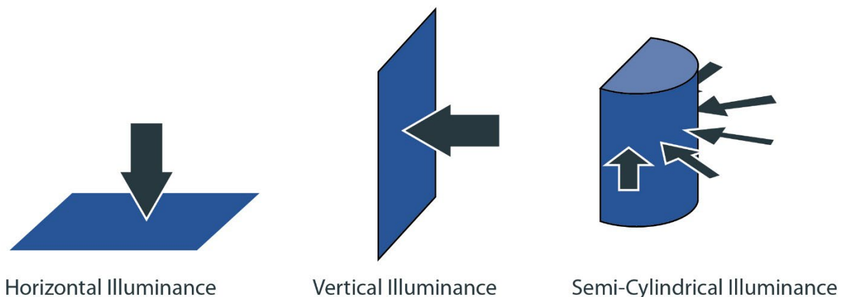
Figure 12. Diagram. Schematic showing the three aspects of illuminance.( Image Credit: VTTI)
