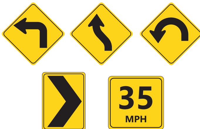
Figure 3. Top row: three advanced curve warning signs. Bottom Row: Chevron sign and advisory speed plaque.
