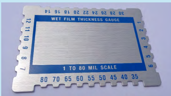
Figure 7. Photograph. Wet film thickness gage used to measure resin binder thickness during application.
