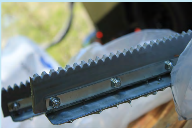
Figure 13. Photograph. Notched rubber squeegee for spreading resin binder during manual application.
