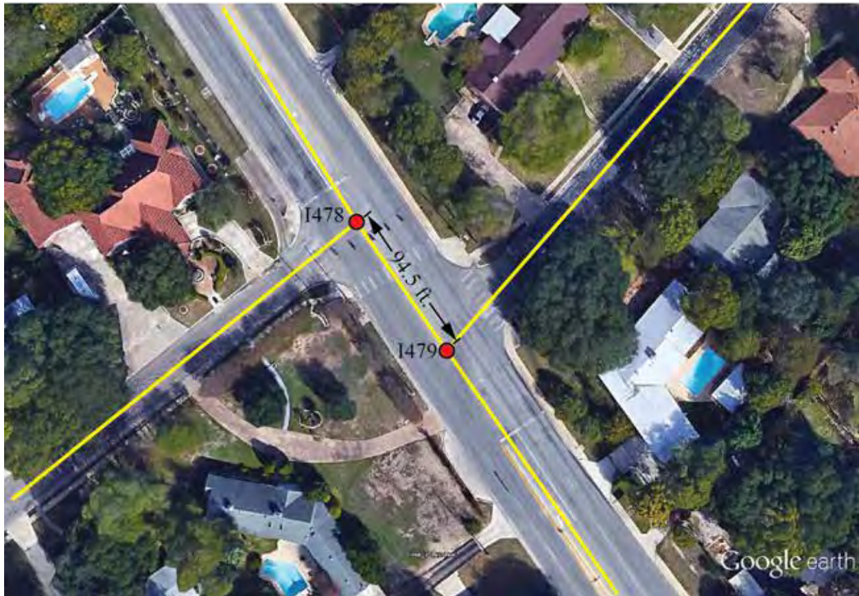
Figure 25. Intersection Offset Distance Measurement.
