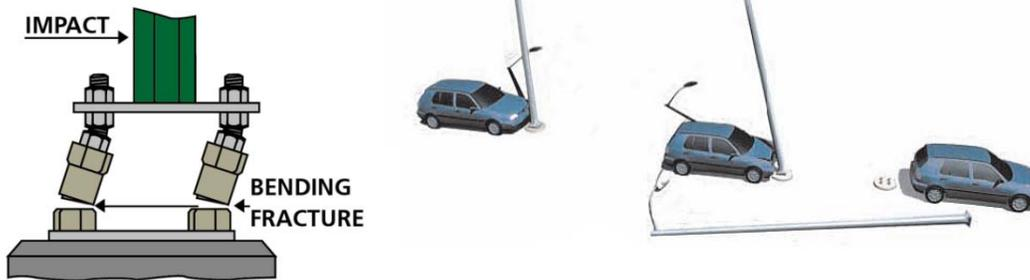
Figure 39 – Pole with Breakaway Device
