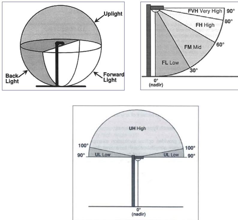
Figure 27 - Lamp Lumen Zones and Front Light Zone (from IESNA TM-15)
