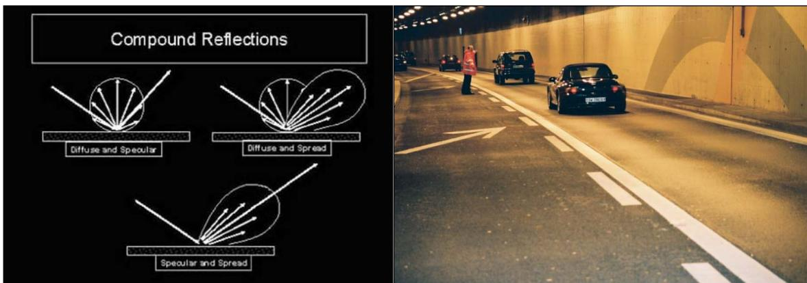
Figure 16 - Pavement Reflective Differences
