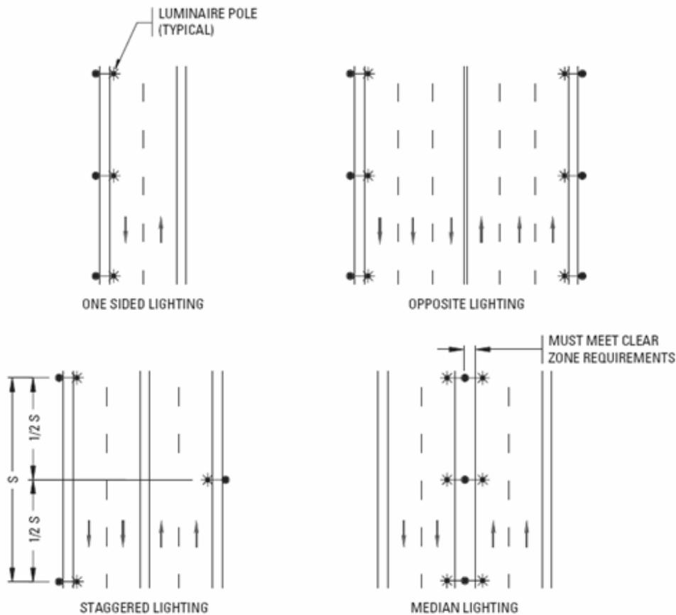
Figure 31 – Typical Pole Spacing
