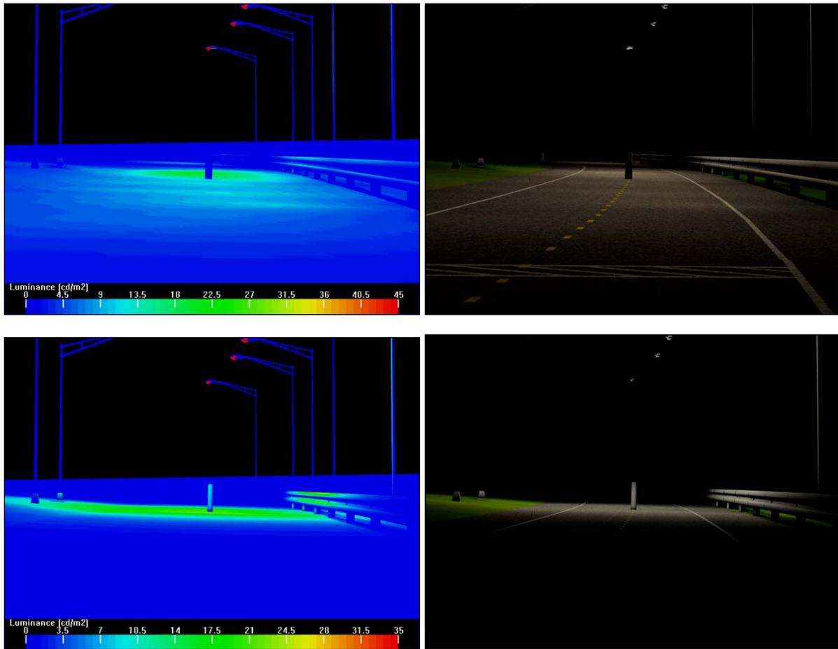
Figure 6 - Luminance Contrast (negative contrast above and positive below)
