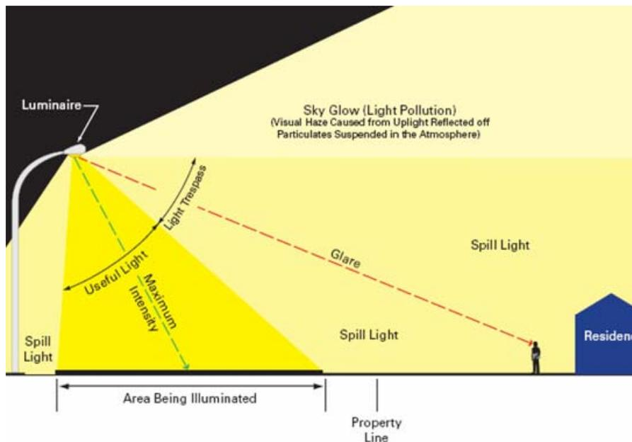
Figure 18 – Spill Lighting, Glare and Skyglow
