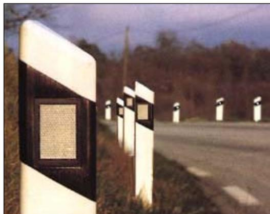
Figure 41 – Post-Mounted Delineators (PMDs)
