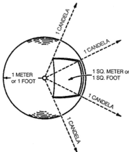
**Figure 2 - Relationship between candelas, lumens, lux, and footcandles:**
