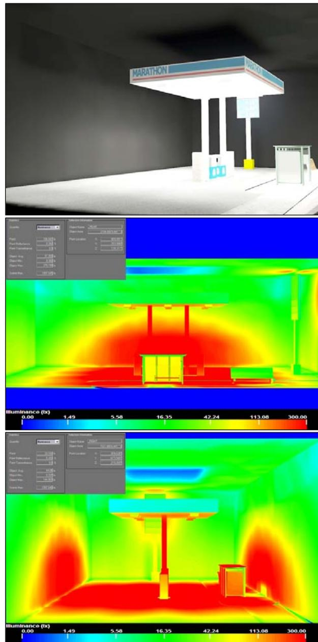
Figure 35 - Example Calculation of Lighting on Surfaces of Theoretical Box
