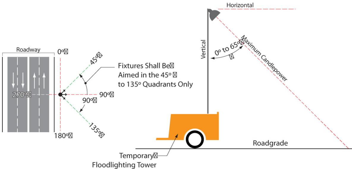
Figure 44 – Work Zone Floodlight Aiming
