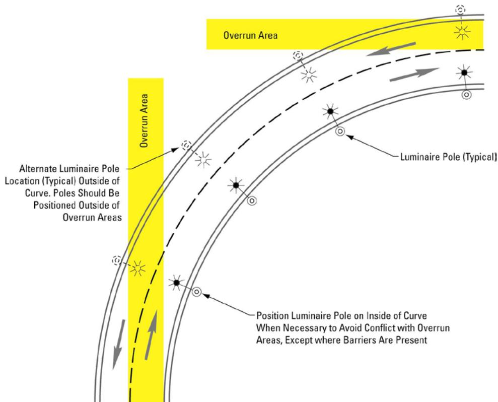
Figure 38 – Pole Spacing on Curves
