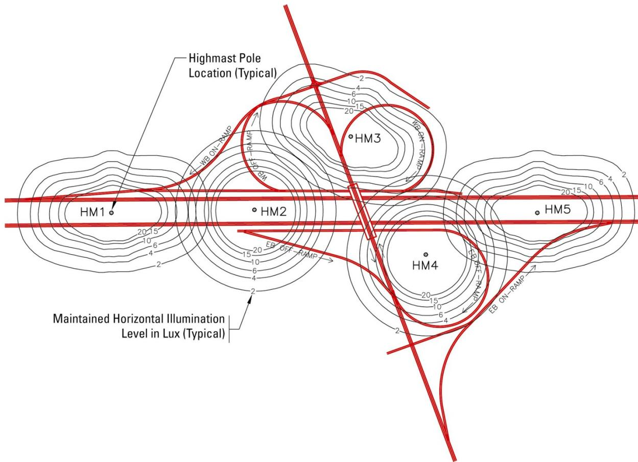
**Figure 33 - Highmast Pole Spacing**
