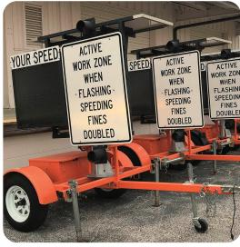
AWAD installed on portable trailers ready for deployment to work zones. Photo courtesy FDOT.
