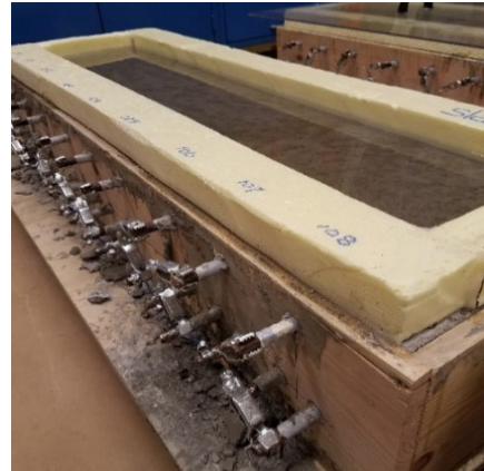
Figure 2. Photograph. Specimen undergoing chloride ponding, with solution being held in place by a foam dam.
