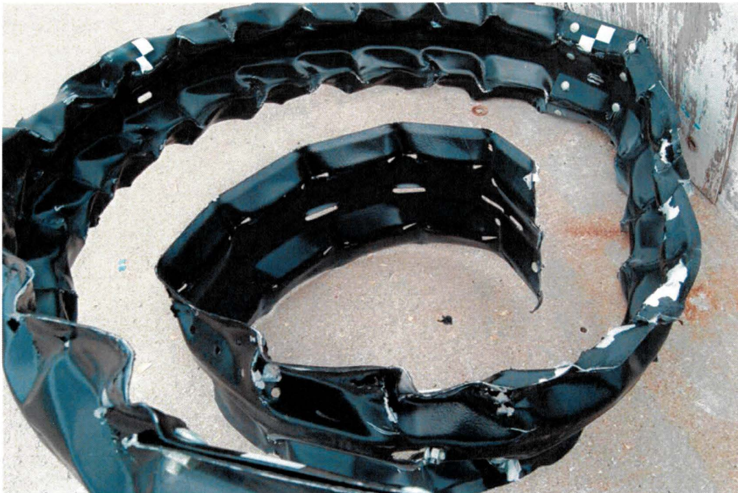
Figure 3. Photograph Showing Kinked Rail
