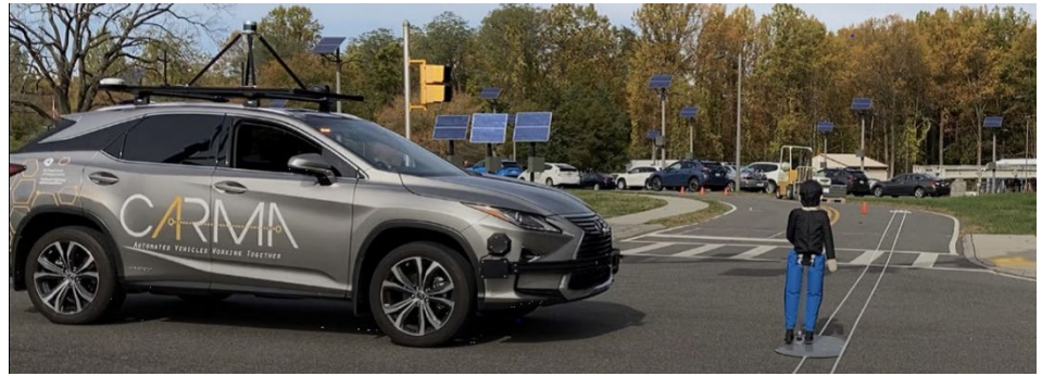
Figure 4. The Human Factors Team testing detection of an articulated child pedestrian dummy.
