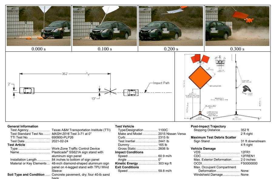
Figure 6.6. Summary of Results for *MASH* Test 3-71 at 0 Degrees on Plasticade® SS621A Sign Stand with Aluminum Sign Panel Mounted at 84 inches.
