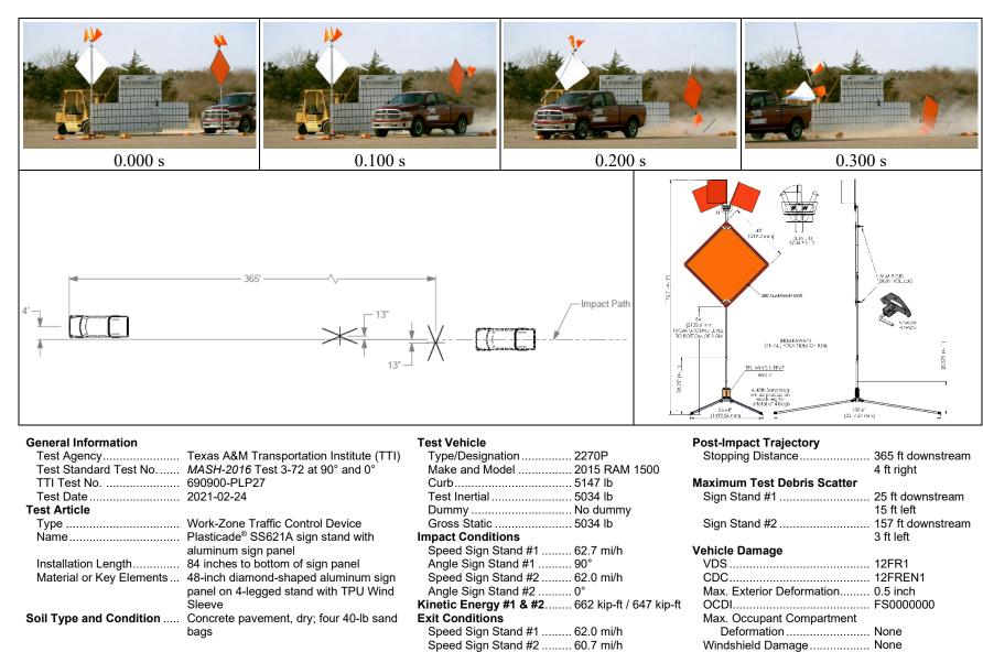
Figure 7.6. Summary of Results for *MASH-2016* Test 3-72 at 90 Degrees and 0 Degree on Plasticade® SS621A Sign Stand with Aluminum Sign Panel Mounted at 84 inches.
