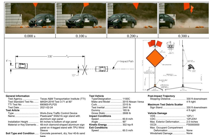
Figure 5.6. Summary of Results for *MASH-2016* Test 3-71 at 90 Degrees on Plasticade® SS621A Sign Stand with Aluminum Sign Panel Mounted at 84 inches.
