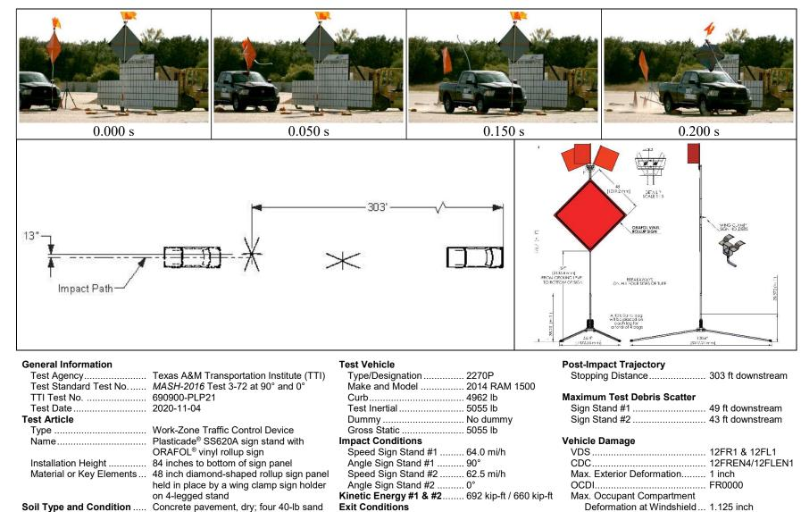
Figure 7.6. Summary of Results for *MASH-2016* Test 3-72 at 90 degrees and 0 Degrees on Plasticade® SS620A Sign Stand with Rollup Sign at 84 inches.
