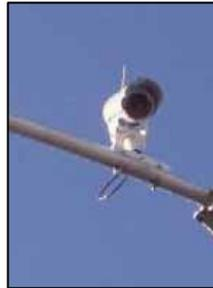
**Figure 24. Camera Used for Automated Pedestrian Detection**
