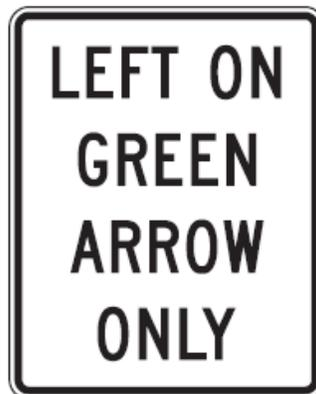
**Figure 35. Static Sign Supporting the Prohibition of Permissive Left Turns**
