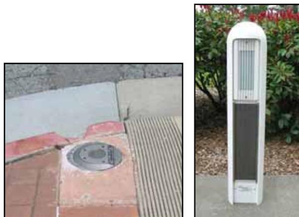
**Figure 27. In-surface (Left) and Above Ground Bollard (Right) Sensors Used in San Francisco**
