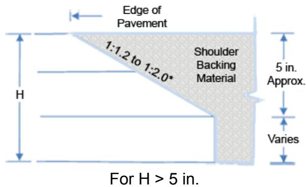
*Note 1\*: Recommended Rise to Run ratio range 1:1.2 to 1:2.0. The range of slope is equal to 26° to 40°.*
