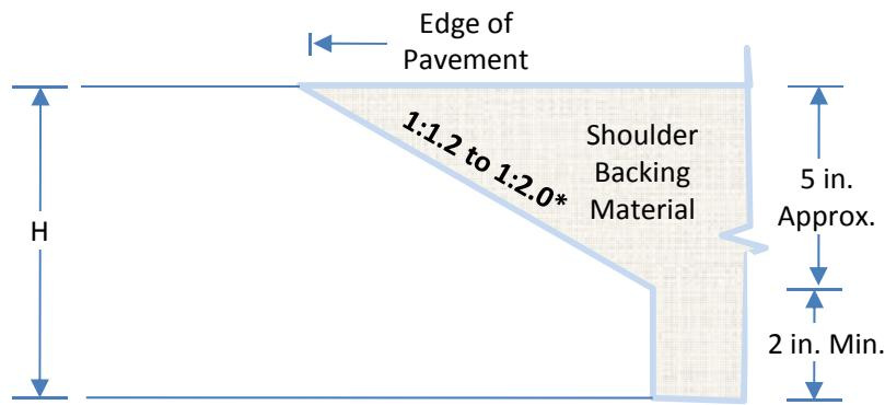
*Note 1\*: Recommended Rise to Run ratio range 1:1.2 to 1:2.0. The range of slope is equal to 26° to 40°.*
