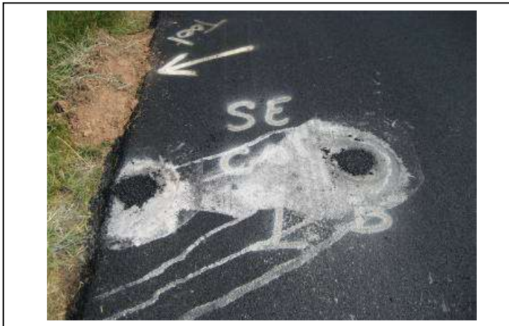
Core #1; Safety Edge SM section (A location is adjacent to the Edge; B location is near the center of the steel drum roller (about 3 feet from edge).
