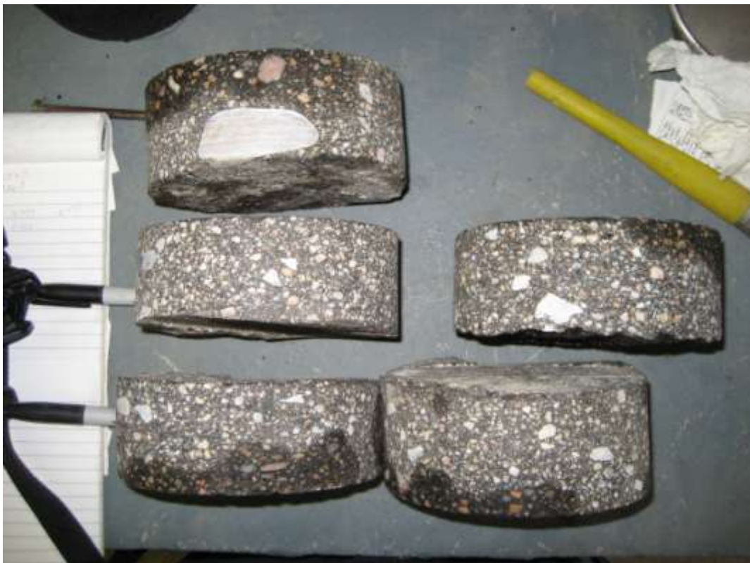
Figure A-1. Cores recovered for laboratory density testing.
