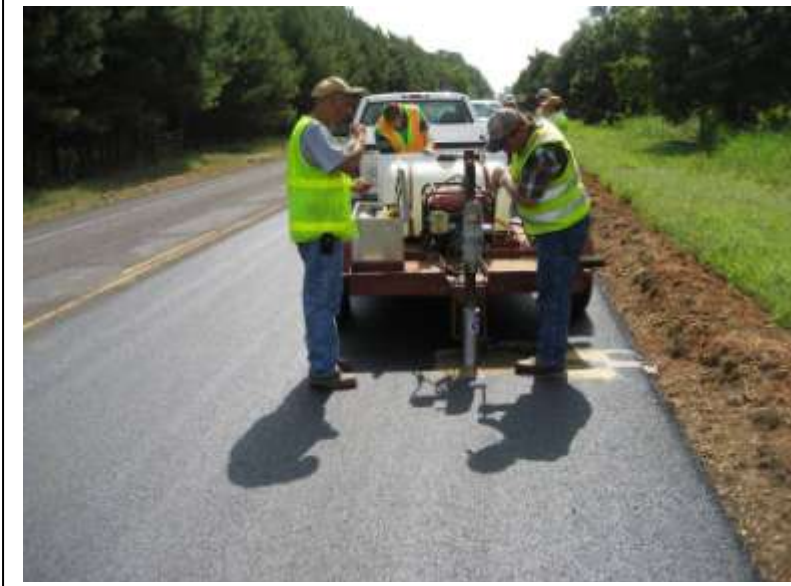
Figure 9. Photos showing location of cores and nuclear density tests made with the Troxler 3440 gauge (nuclear density readings were taken and then the HMA overlay was cored).
