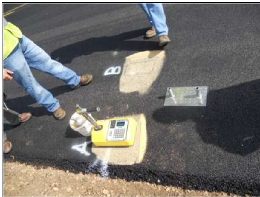
Figure 7. Nuclear gauge used to measure HMA density.
