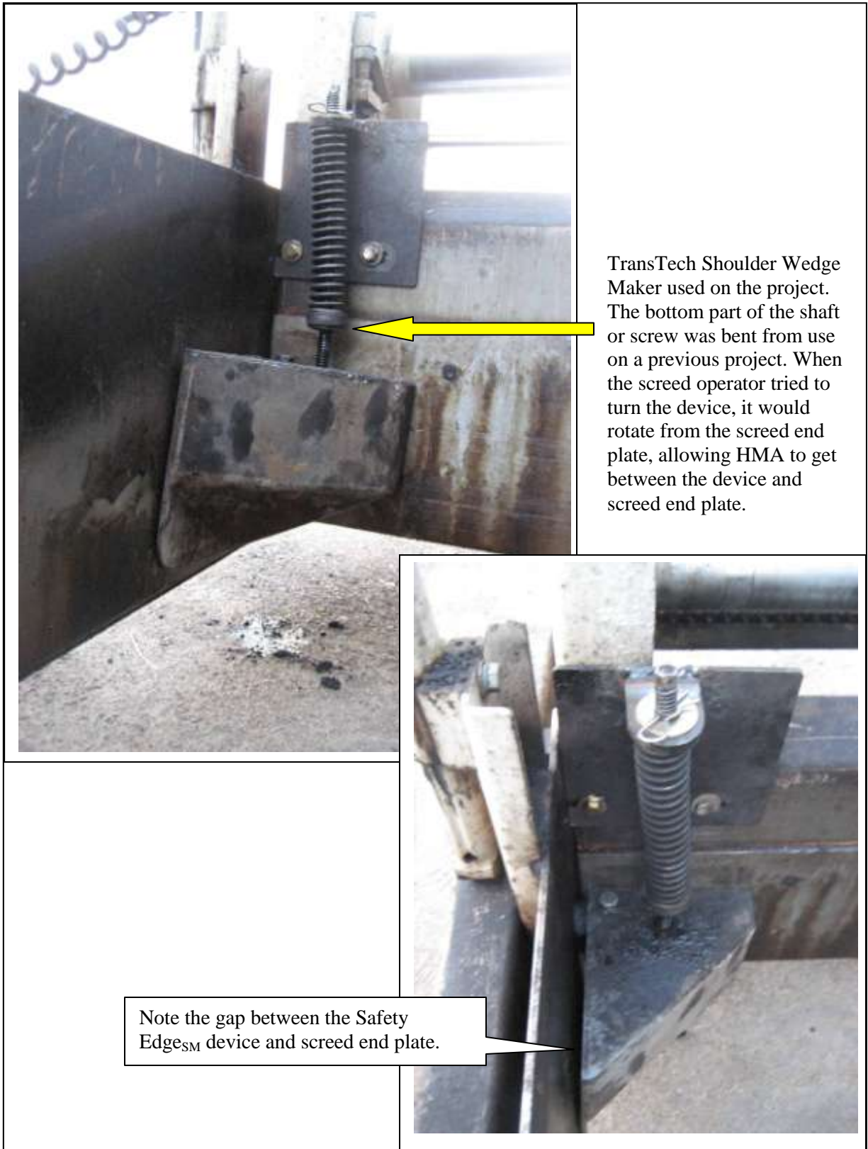
Figure 16. TransTech Shoulder Wedge Maker attached to the screed.
