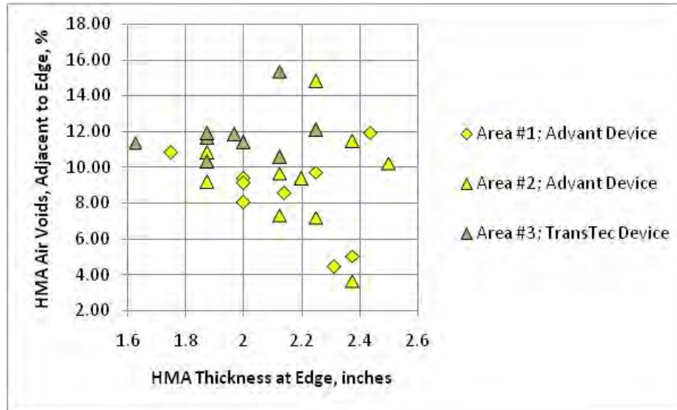
Figure 14. Comparison of WMA thickness at the edge of the mat and WMA air voids.
