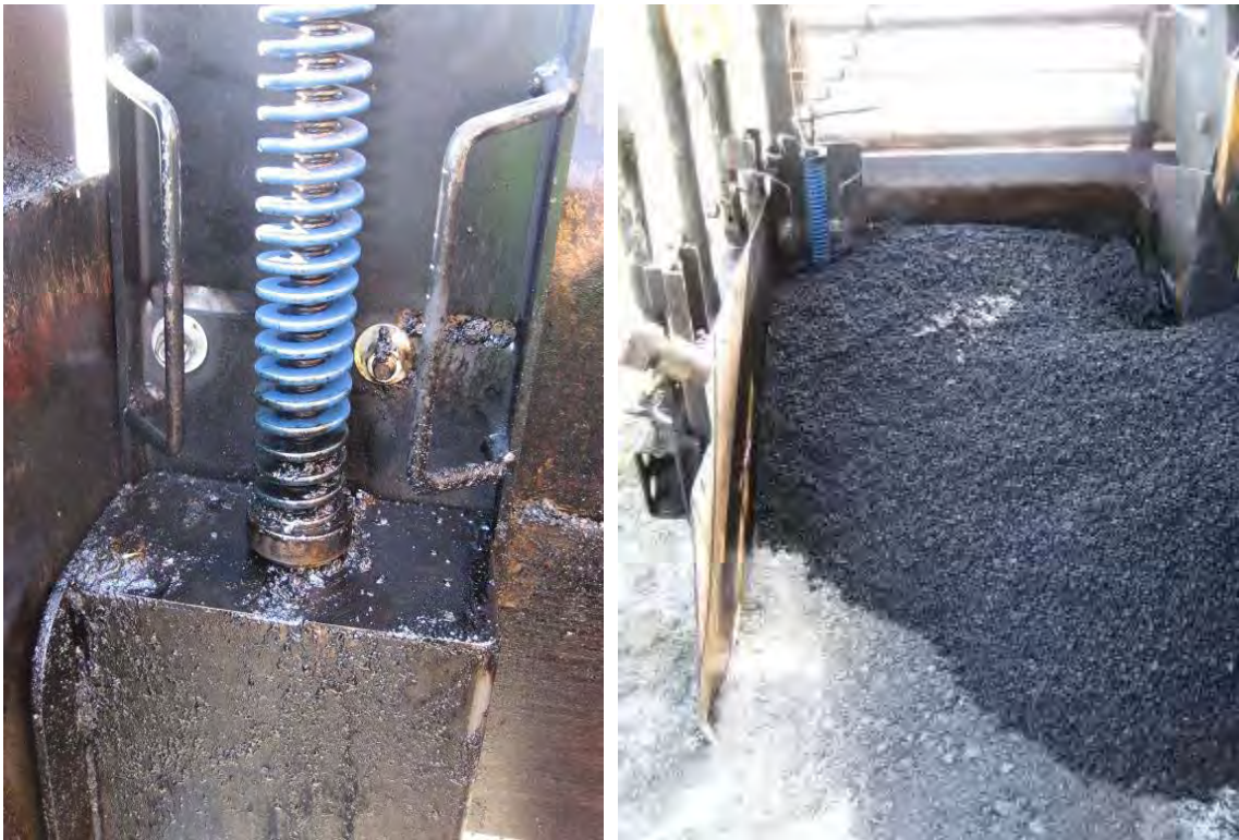
Figure 16. Advant-Edger device attached to the screed.
