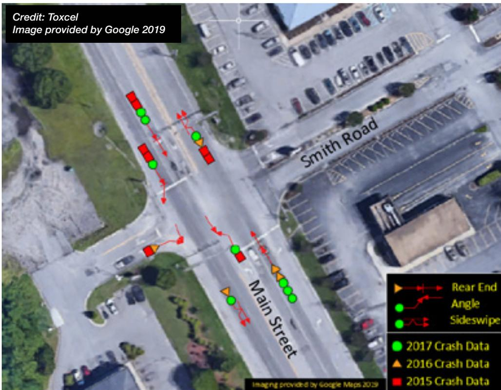
Figure 9: Collision Diagram (2015-2017)
