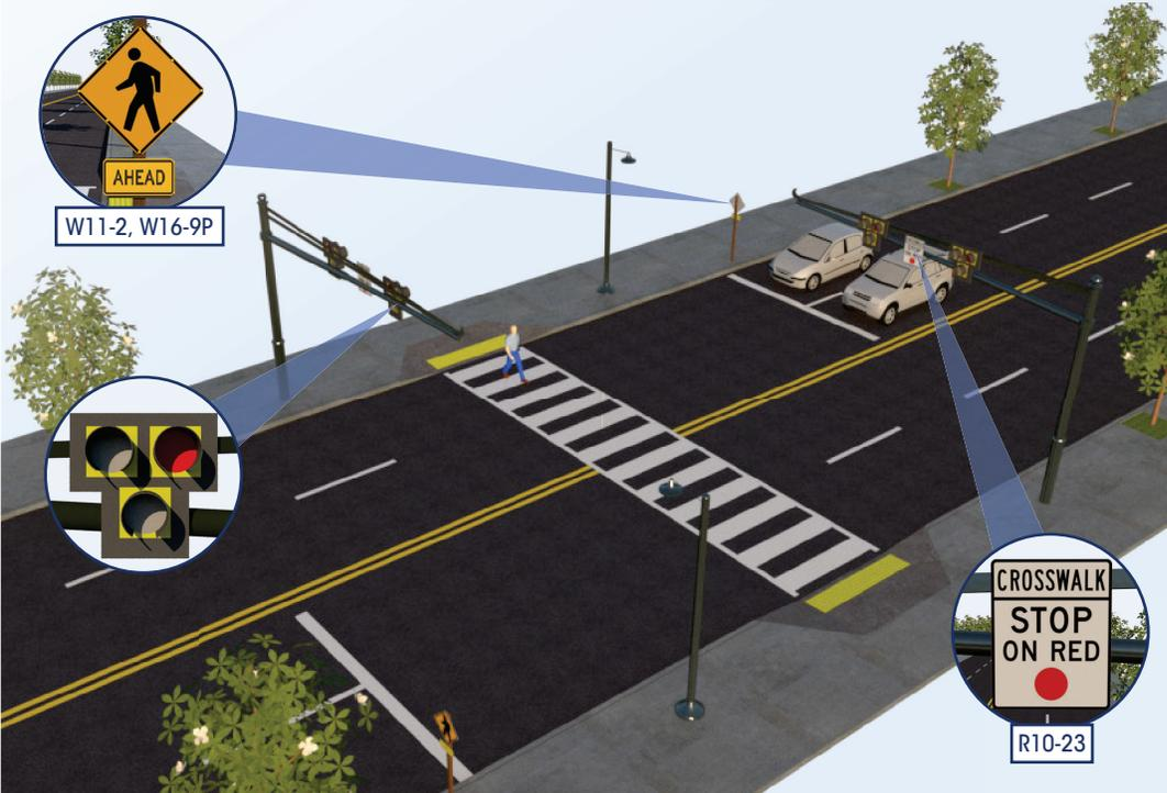
A Pedestrian Hybrid Beacon head consists of two red lenses above a single yellow lens. Unlike a traffic signal, the PHB rests in dark until a pedestrian activates it via pushbutton or other form of detection. When activated, the beacon displays a sequence of flashing and solid lights that indicate the pedestrian walk interval and when it is safe for drivers to proceed (see figure on back page).
