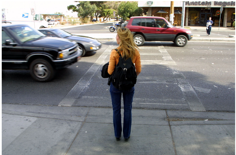
As vehicle speeds and volumes increase, so does the complexity of a pedestrian's crossing. Crosswalks alone may not be sufficient to facilitate vehicle yielding. Credit: Dan Burden, PBIC Image Library.
