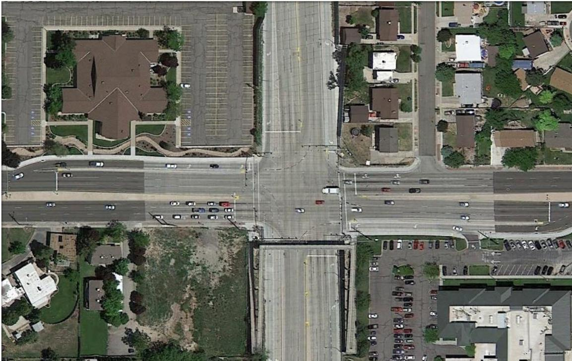
**Exhibit 1-3. Four-legged DLT intersection with four displaced lefts (West Valley City, UT).<sup>(1)</sup>**
