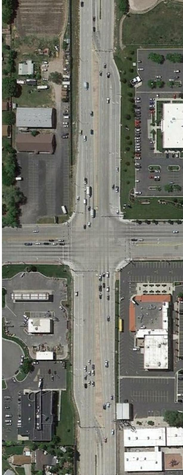
**Exhibit 7-7. Four-legged DLT intersection with major street displaced left turns and without channelized right turns (West Valley City, UT).<sup>(1)</sup>**
