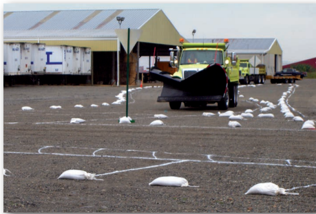
Figure 2: A snow plow approaching the mock roundabout.
