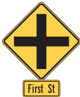
Figure 19. Intersection Warning W2-1 Sign and W16-8P Supplemental Advance Street Name Plaque
