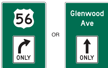
Figure 34. Combination Lane Use/Destination Guide Sign (MUTCD D15-1)
