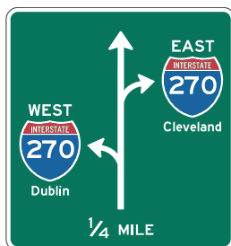
Figure 45. Advance ground-mounted diagrammatic sign
