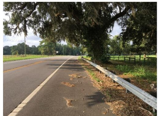
Guardrail shielding large tree. Source: FHWA
