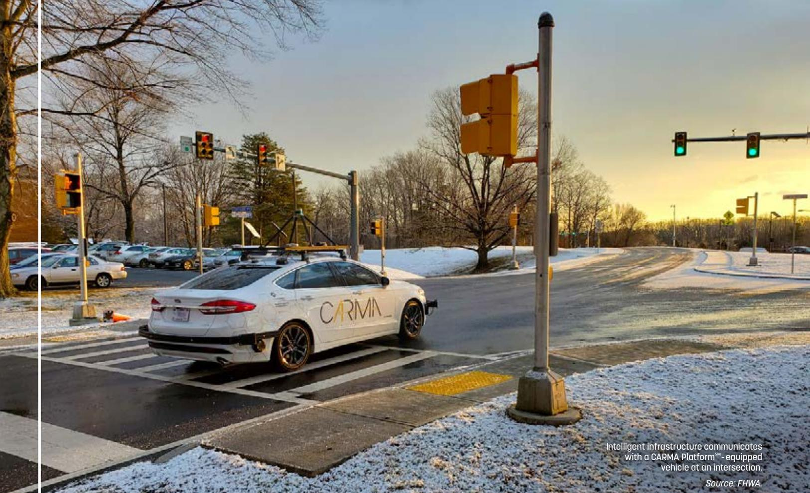
Intelligent infrastructure communicates with a CARMA Platform<sup>SM</sup>-equipped vehicle at an intersection.
