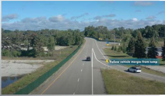
CARMA Platform-equipped vehicle merges onto a freeway during validation testing.
