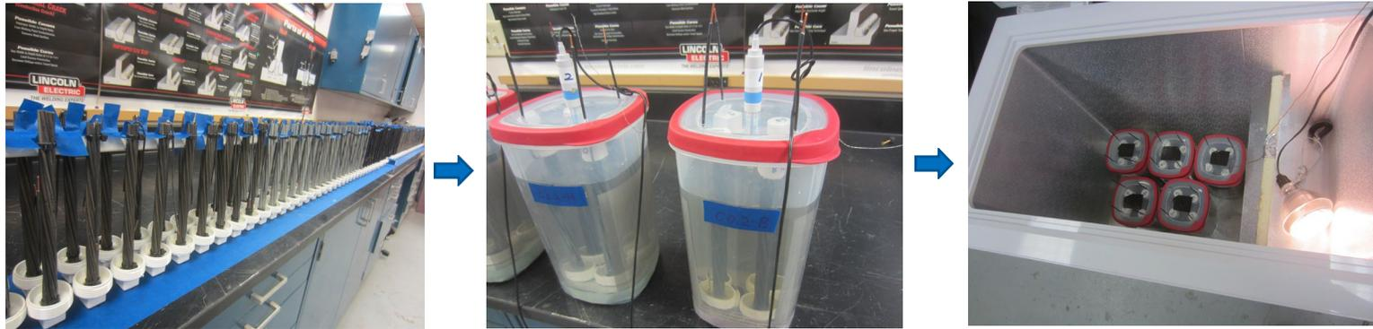
Corrosion resistance testing in simulated pore water and bleed water
