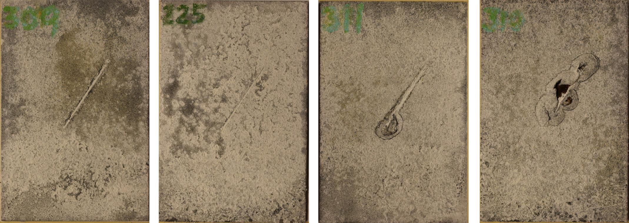
Aluminum-zinc coated panels showing coating failure after 10 ALT cycles
