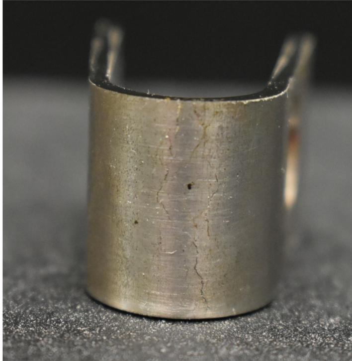
SCC in 316LN SS due to magnesium chloride
