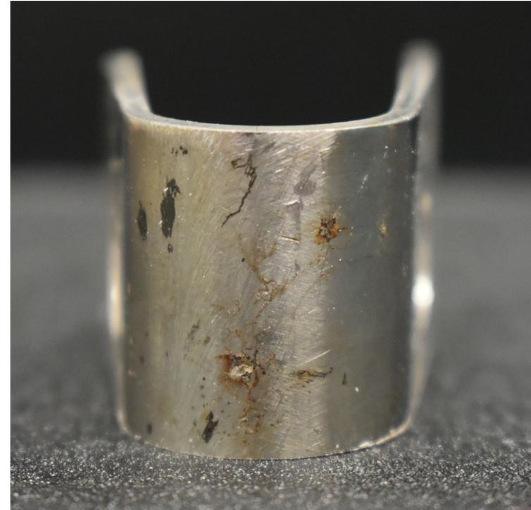
SCC in 304L SS due to calcium chloride
