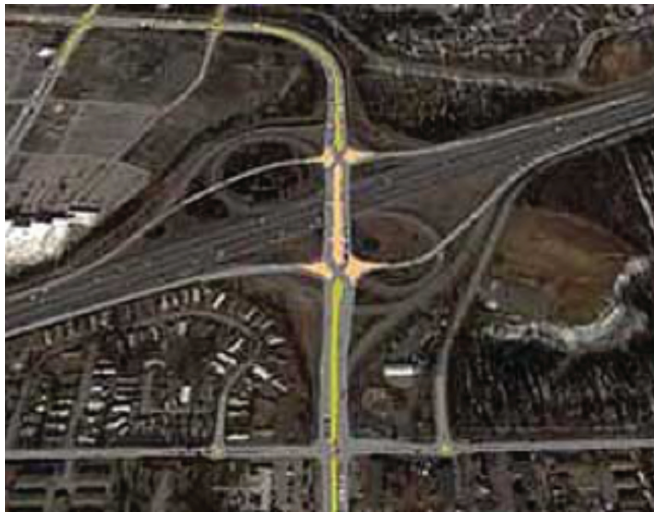
An aerial view of a two-cloverleaf highway interchange from a simulation video created by Nopadon Kronprasert. © Wei Zhang, Nopadon Kronprasert, and Jason Williams.
