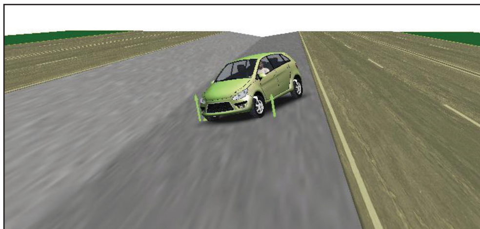
A simulation model for investigating vehicle behavior on a sloped terrain surface. Source: FHWA.
