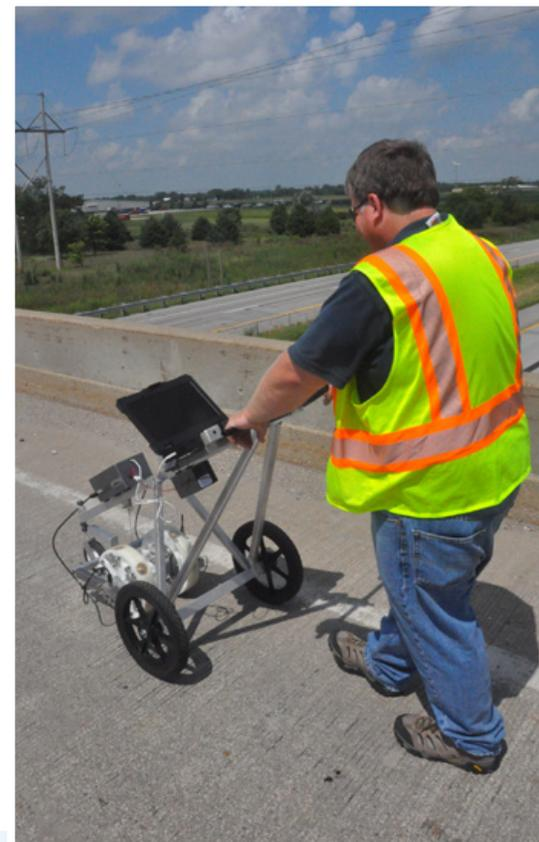
A bridge inspector uses a cart-based impact echo system on a bridge deck in Iowa.
