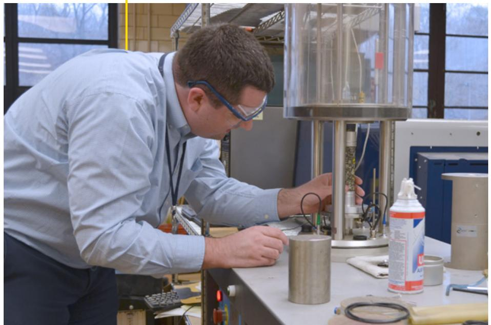
Rafic El-Helou installs sensors to measure the deformation of a UHPC beam in FHWA's Structures Laboratory.
