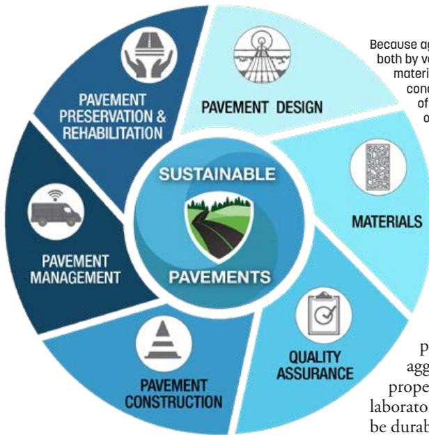
Because aggregates are the predominant constituent, both by volume and mass in the various pavement materials and layers (bases, asphalt, and concrete), the selection and quality assurance of aggregates play a major role in all segments of the pavement life cycle wheel.
