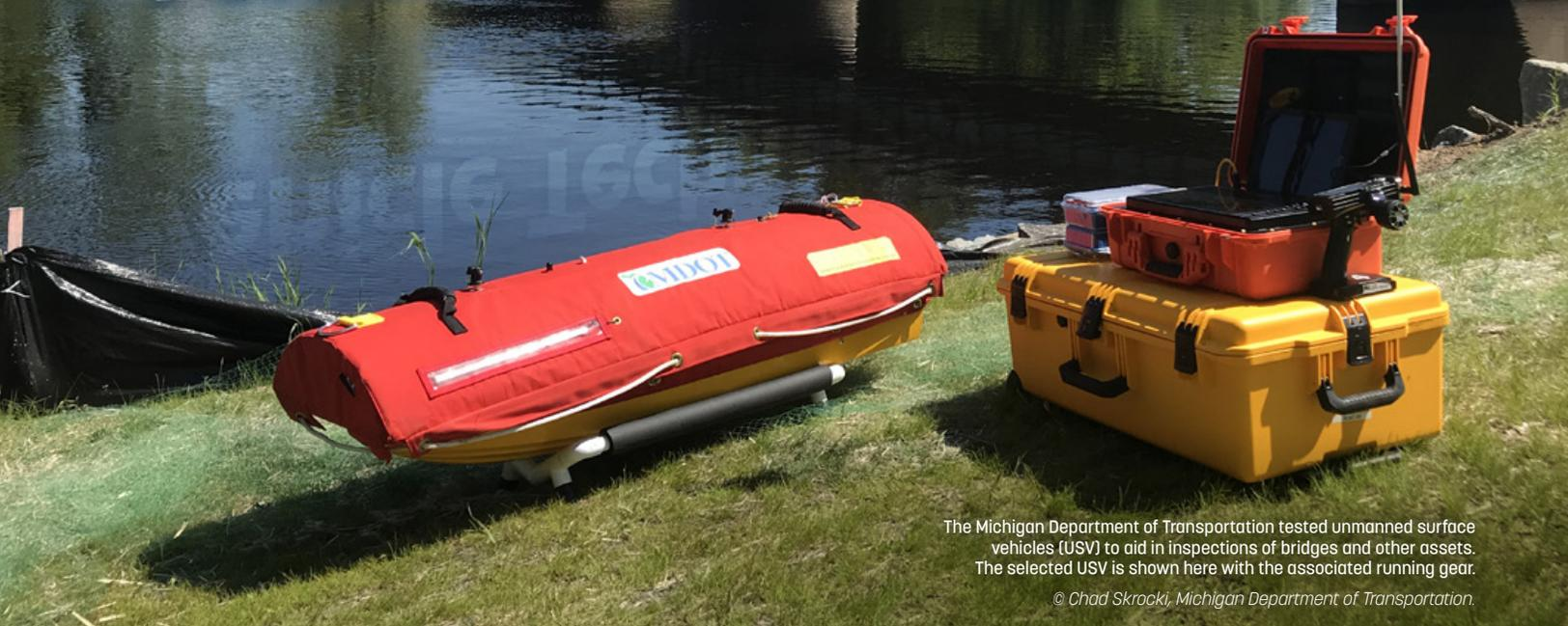
The Michigan Department of Transportation tested unmanned surface vehicles (USV) to aid in inspections of bridges and other assets. The selected USV is shown here with the associated running gear.
