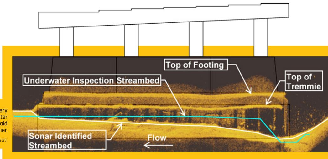
The research team compared sonar imagery collected using MDOT's USV to the underwater inspection streambed performed by divers, overlaid on a drawing of the elevation of the pier.
