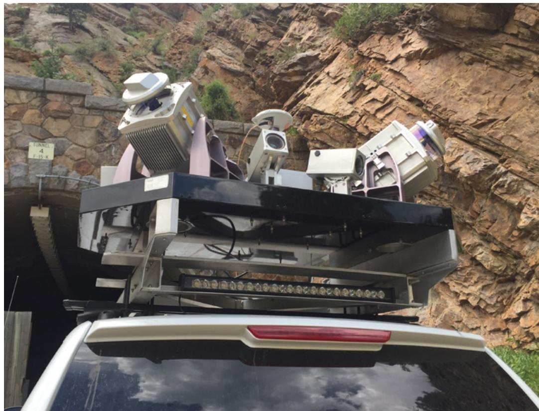
CDOT used this truck-mounted high-speed IR and LiDAR system in tunnel inspections.
