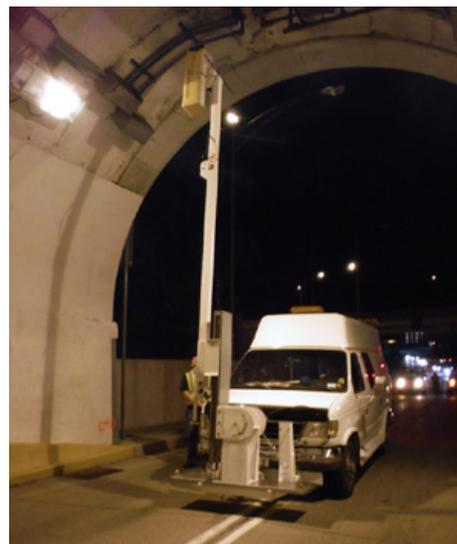
PennDOT used this van-mounted GPR system to inspect tunnel walls.
