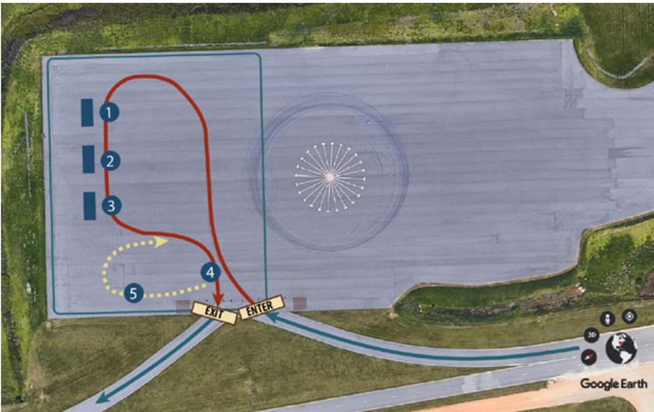
This map shows a proposed use case test route for port drayage at a test track. The commercial motor vehicle enters, is directed to one of three loading points (1, 2, 3), goes through a virtual inspection point (4), and then exits if it passes inspection or proceeds to a holding area (5) if it does not.
