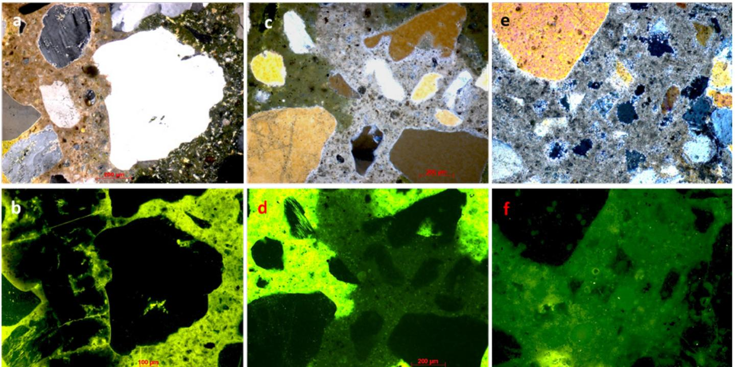
Photomicrograph of thin sections of recycled concrete aggregate particles for analysis, viewed through a petrographic microscope. The top images use cross-polarized light for mineral identification. The bottom images use fluorescent light to study porosity.
