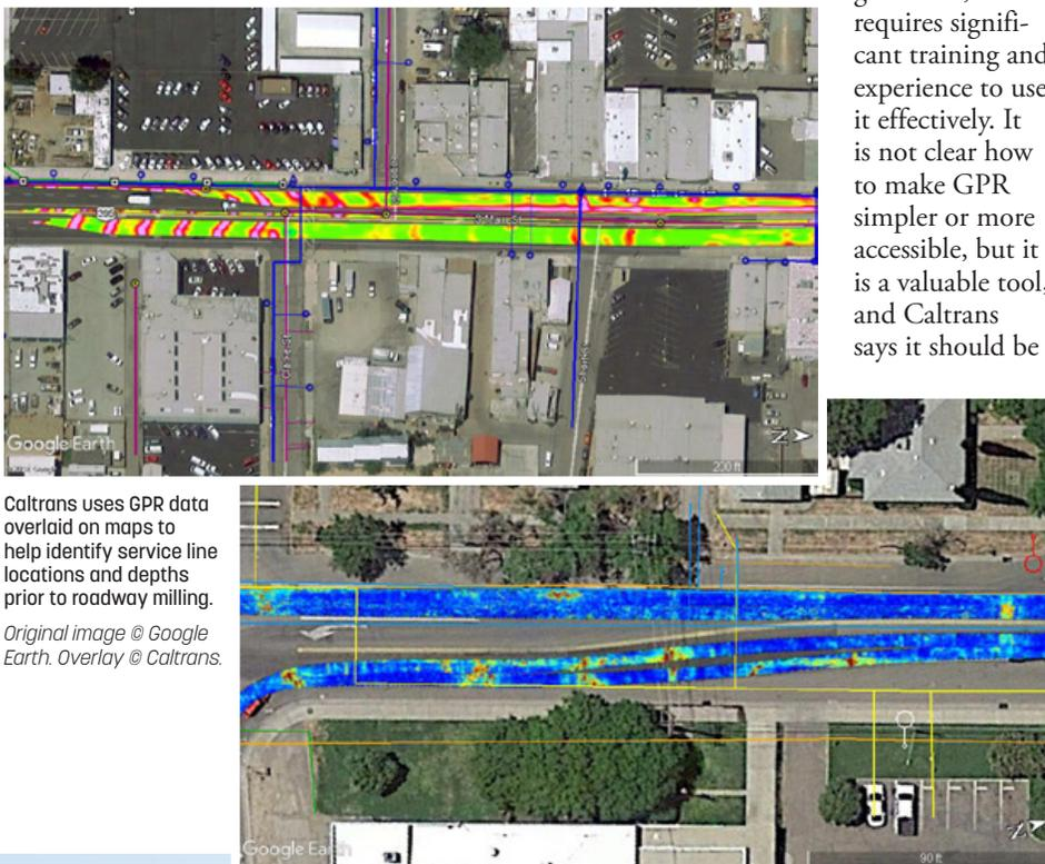
Caltrans uses GPR data overlaid on maps to help identify service line locations and depths prior to roadway milling.
