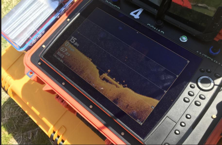
Sonar imagery showing a pier footing displays in real time on the USV operator's equipment in the field.
