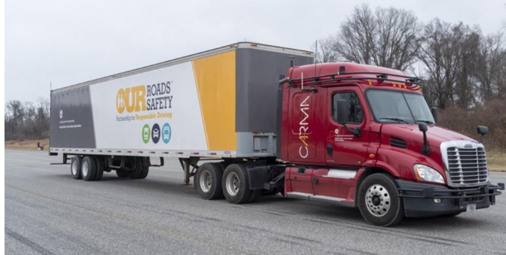
CARMA-equipped vehicles like this truck are helping FHWA, MARAD, and FMCSA discover how CDA technologies can improve safety and efficiency for commercial freight.
