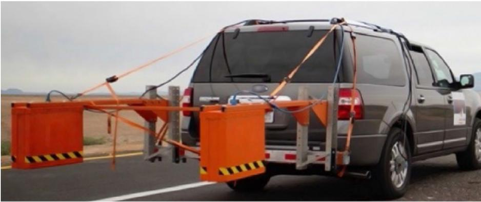
The Nebraska Department of Transportation uses a truck-mounted, air-coupled GPR system to evaluate bridge decks.
