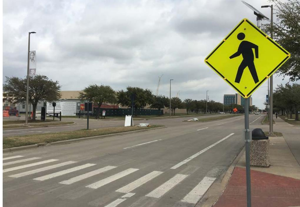
Pedestrian crossing sign with embedded LEDs.
