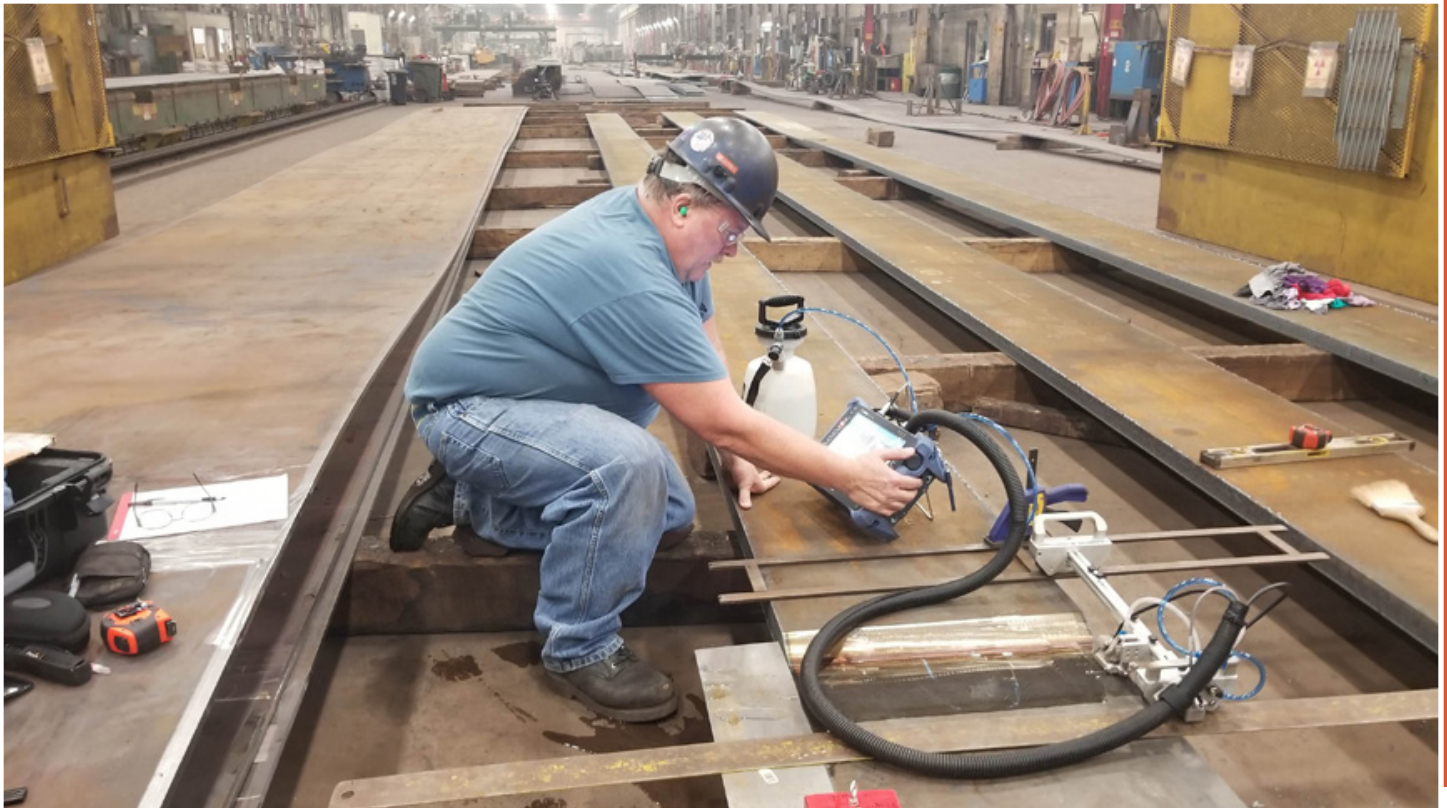
A worker performs an ultrasonic inspection of a weld in a steel fabrication shop.
