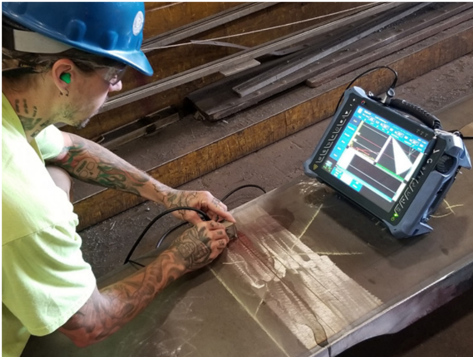
PAUT enables inspectors to capture data and produce images similar to a radiographic image.
