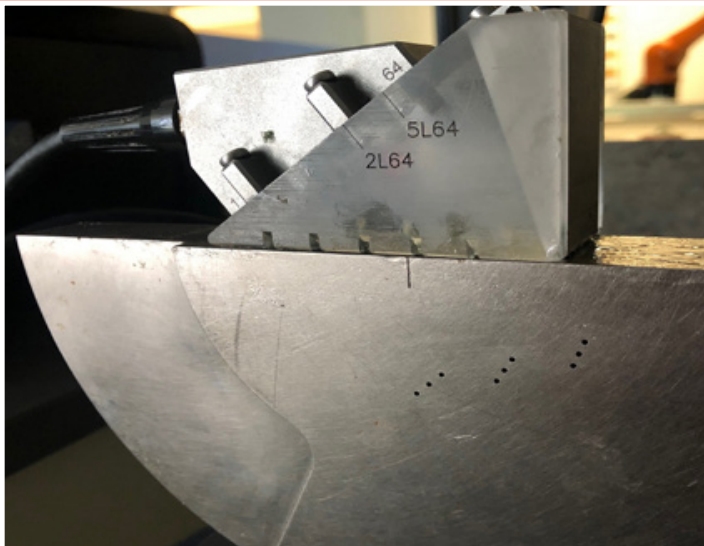
To illustrate the difference in the visual display capabilities of ultrasonic testing methods, FHWA's NDE Lab created this steel block with three sets of three holes with 1-millimeter diameters, and scanned it using different techniques.
