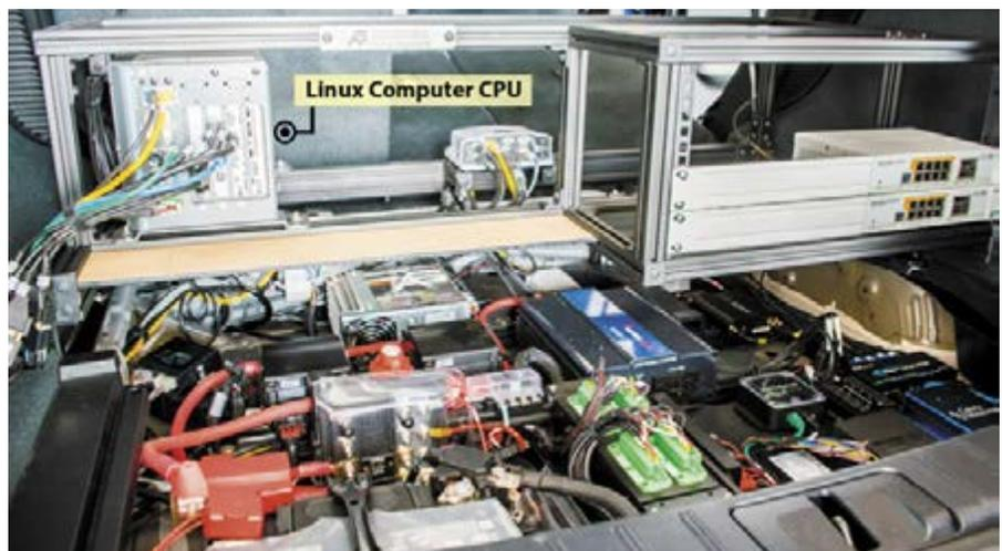
The Linux-based computer housed in the vehicle’s trunk runs the speed and steering software.
