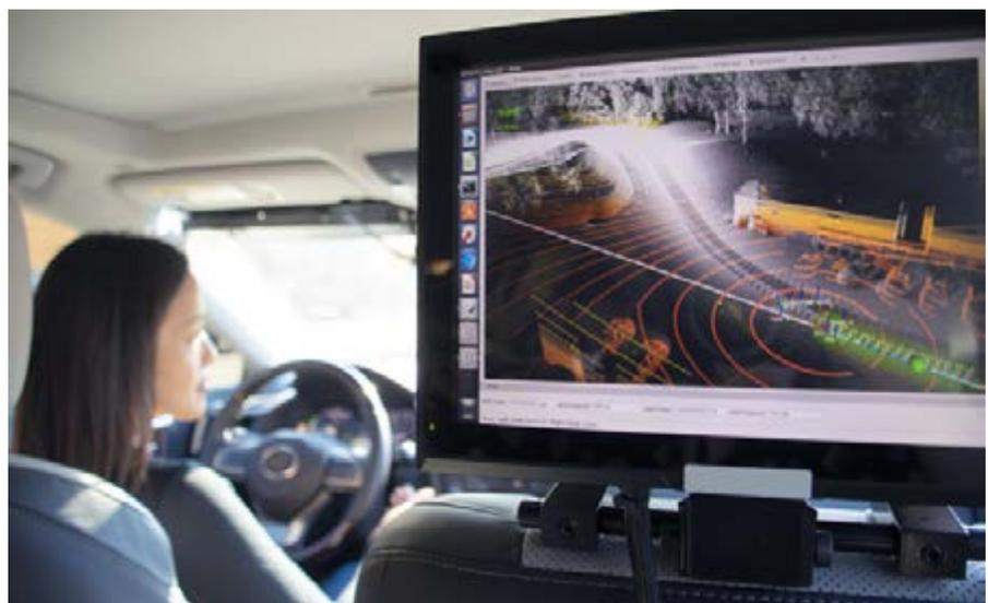
This photo depicts how waypoint following appears on a screen in a CARMA3-equipped vehicle to show localization, which is how CARMA recognizes what is around the vehicle.
