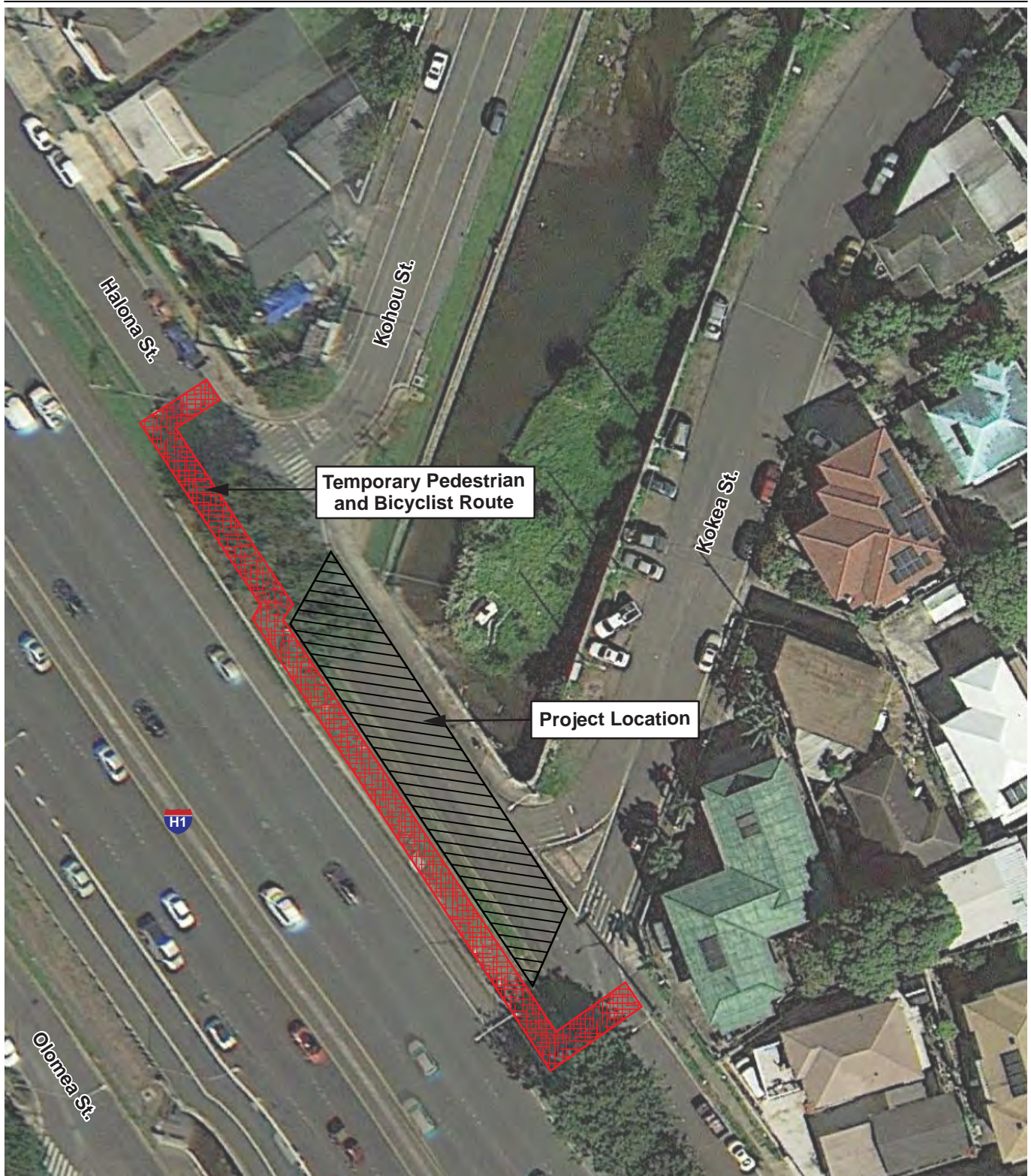
FIGURE 2-7 Temporary Pedestrian and Bicyclist Route During Construction Halona Street Bridge Project Hawaii Bridges Program – Central Federal Lands Highway Division and Hawaii Department of Transportation
